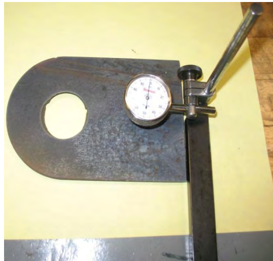
Fig 11. Surface Variation Measurement Tool
