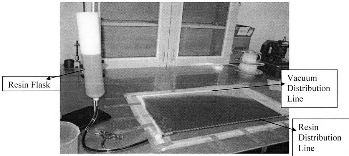
**Figure 2.13: Resin Flow in VARTM Process**
