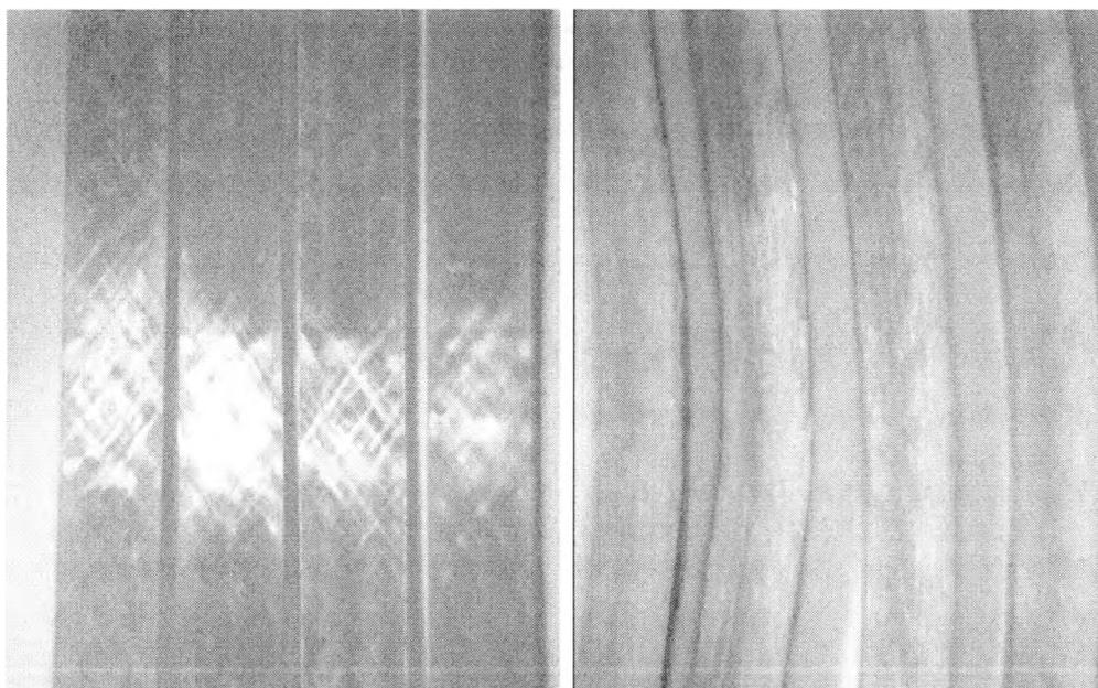
**Figure 4.7: Front and side micrographs of failed flexure specimen**
