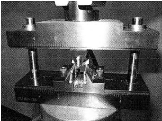
**Figure 3.8 Short Beam Test Fixture Loaded with Specimen**
