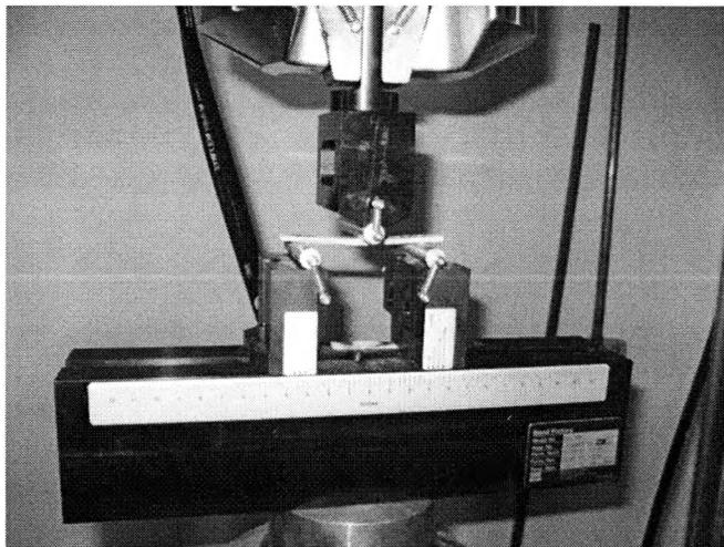
**Figure 3.6 Flexure Test Specimen and Fixture**
