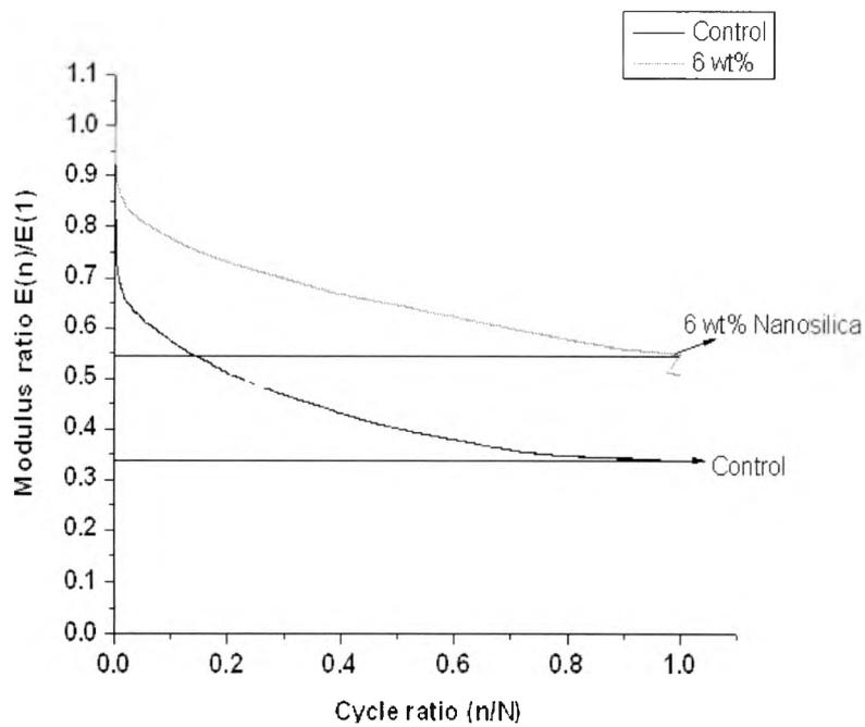
Figure 4.17 Superimposed stiffness degradation curves for 46.6 MPa
