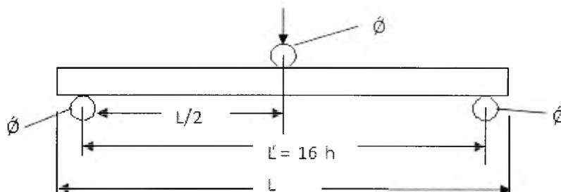
Where  $h$ =thickness, Specimen Length = $L$ , Span Length ( $L^1$ ) = $16h$ , width= $b$
