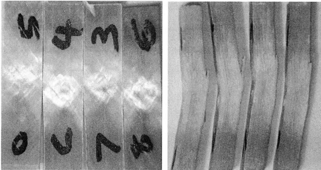
Figure 4.9: Front and side micrographs of failed ILSS specimen
