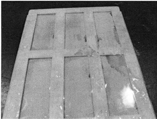
**Figure 2.11: Silicone mold with flexure specimens**
