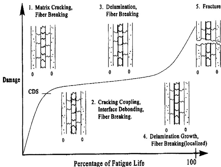
**Figure 1.9: Fatigue Damage Mechanisms in Composite Laminate (Talreja, 1987)**
