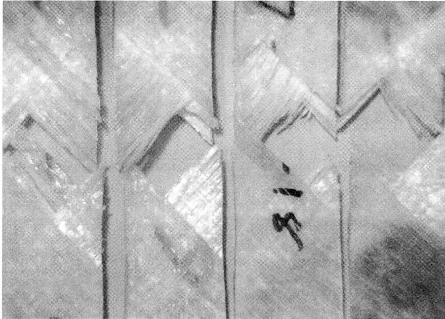
**Figure 4.12: Failed fatigue specimens of control composites at 46.6, 55.9, 65.2, and 74.5 MPa maximum stress**
