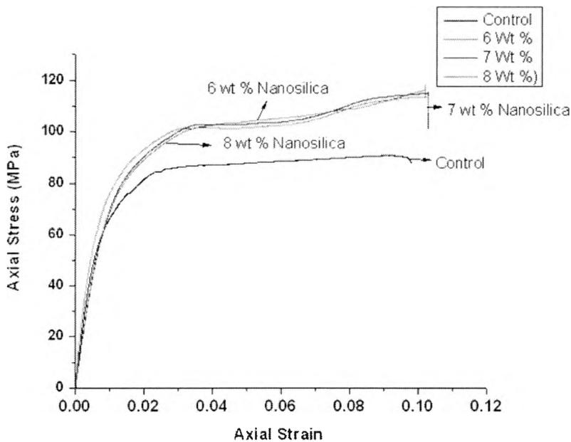
**Figure 4.1: Tensile stress-strain curves for control and nanocomposites**
