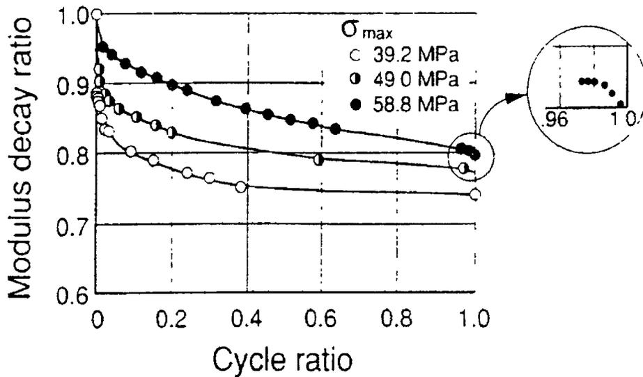
**Figure 1.10: Modulus Decay under Fatigue Loading in Woven Composites**
