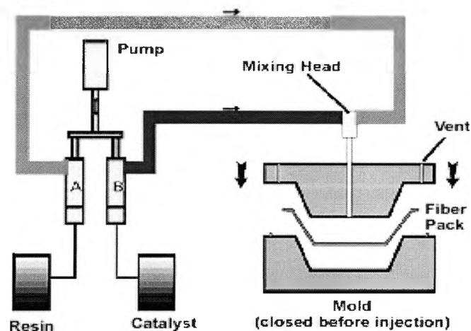
**Figure 2.5 Resin Transfer molding**
