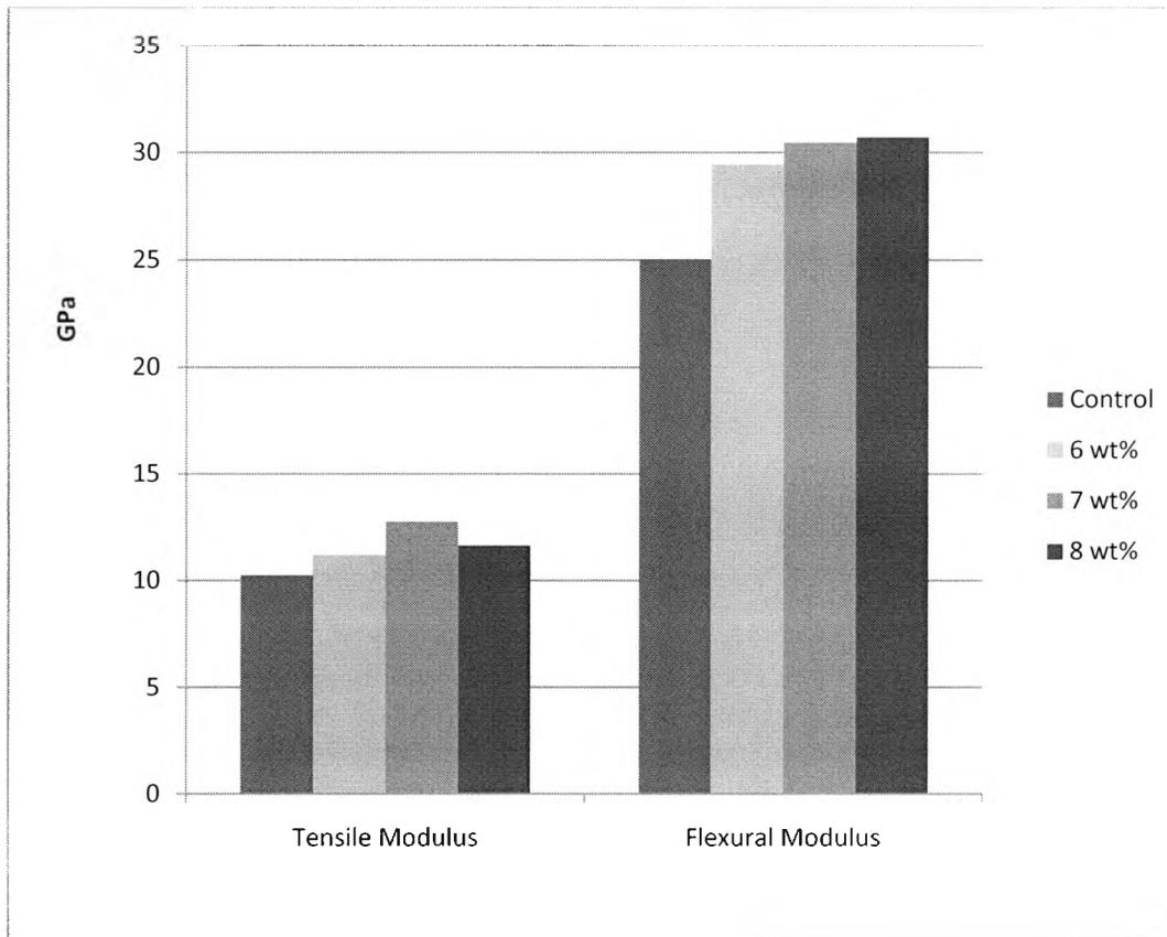
**Figure 4.11: Tensile and Flexural Modulus of control, 6, 7 and 8 wt% Composites**
