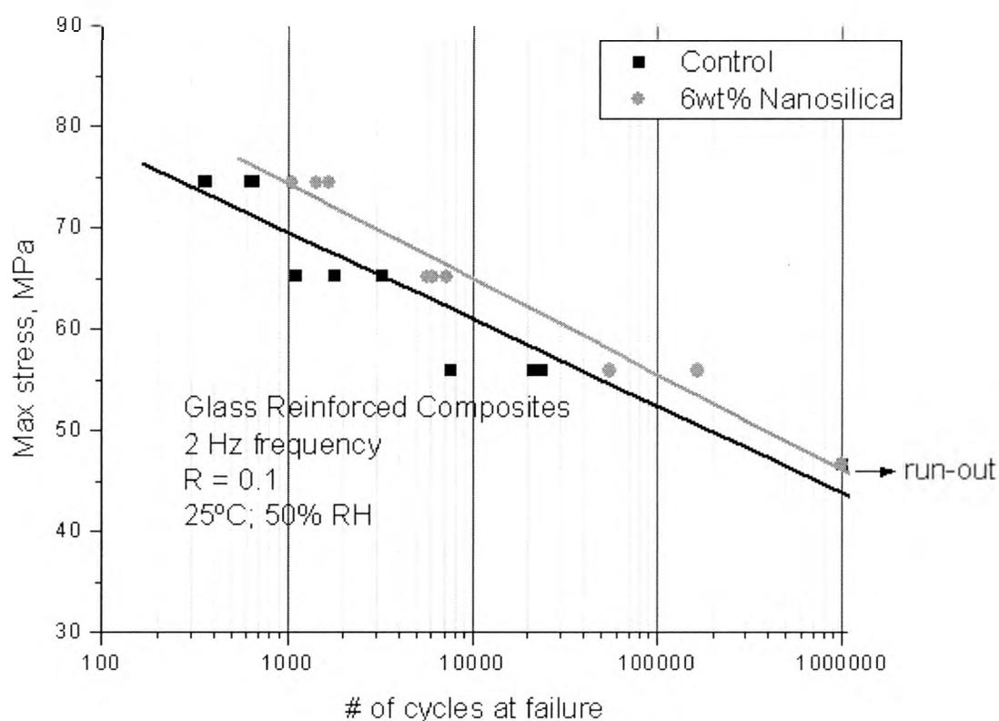
**Figure 4.14: S-N Diagram for Glass reinforced composites**
