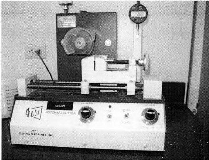
**Figure 3.10: Notching cutter**
