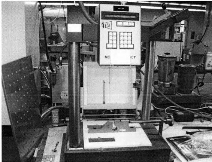
**Figure 3.11: Monitor/ Impact tester**
