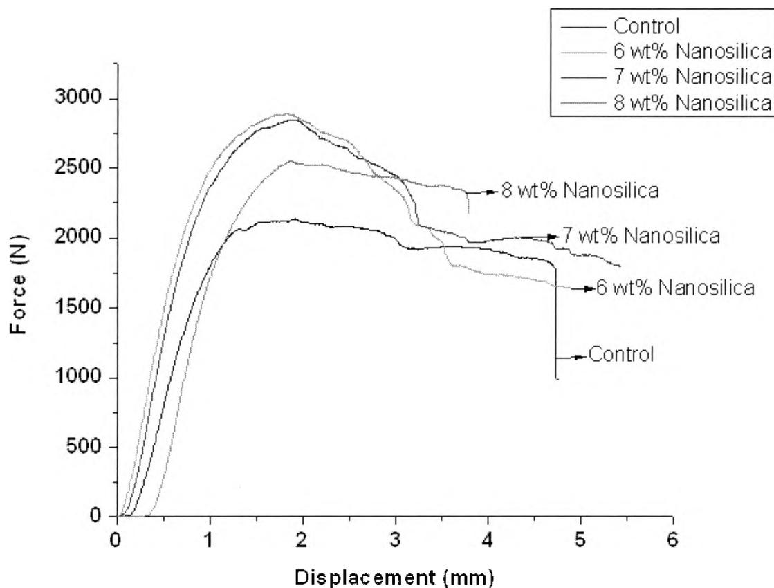
**Figure 4.8: Superimposed load vs cross-head displacement**
