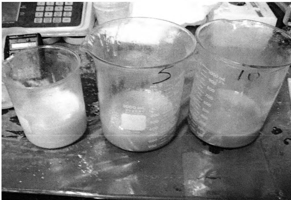
**Figure 4.18: HNT-epoxy mixture after high-shear mixing (2.5wt%, 5wt%, and 10wt% HNT)**
