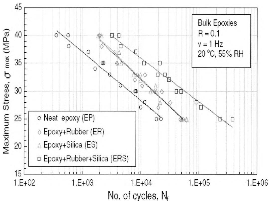
**Figure 4.13: S-N Diagram for Nanomodified Neat Epoxy Resin (Manjunatha, Taylor, Kinloch, and Sprenger, 2009)**
