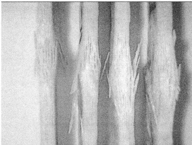
**Figure.4.4: Side micrograph of failed tensile specimen**
