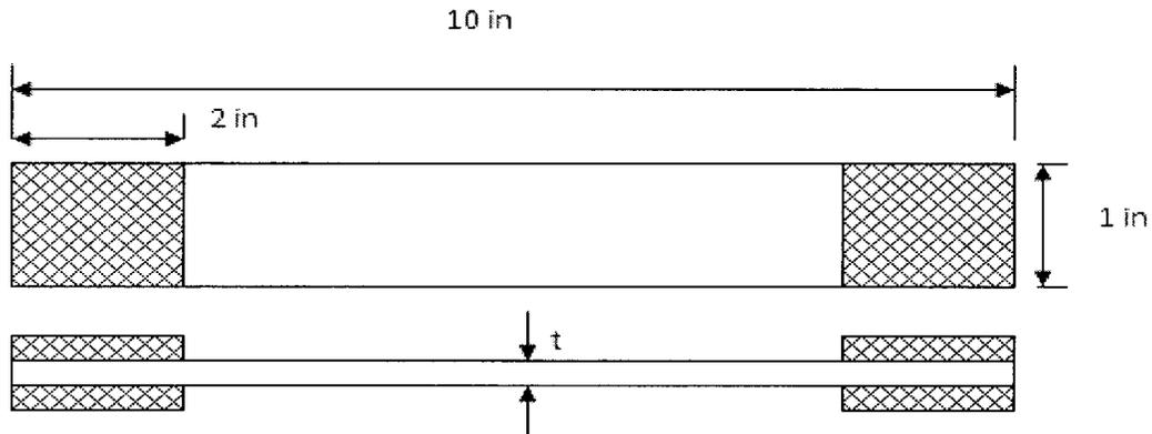
**Figure 3.2 Tensile Tests Specimen**
