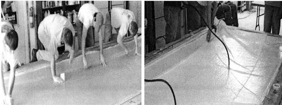
**Figure 2.1: Typical wet layup processing**
