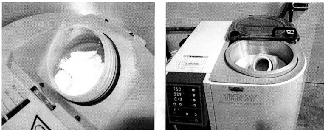
**Figure 2.9: Planetary centrifugal vacuum mixer: Phenolic resin with nanoclay before and after mixing (Kabakov, Tate, Koo, 2010)**
