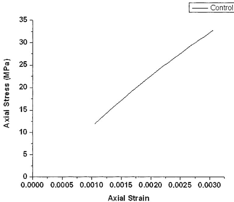
**Figure 4.2: Chord modulus on control specimen**
