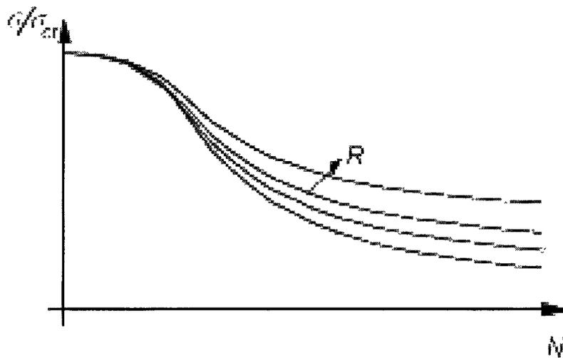
**Figure 1.6 S/N Diagram for different R- values**
