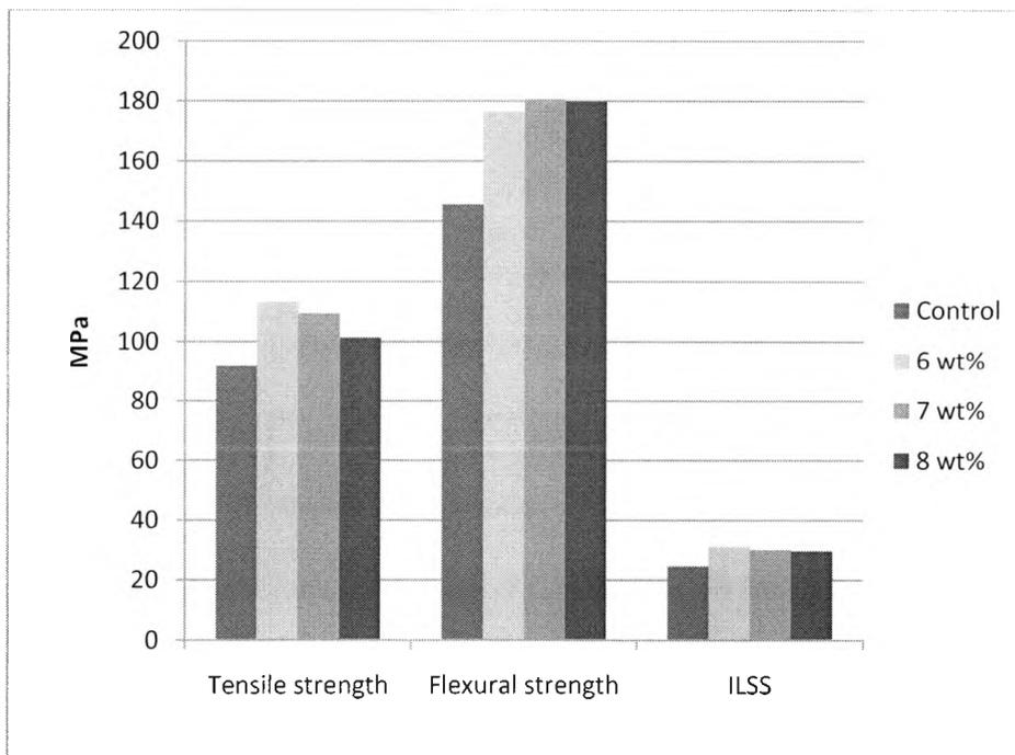
Figure 4.10: Different Strengths of control, 6, 7 and 8 wt% Composites
