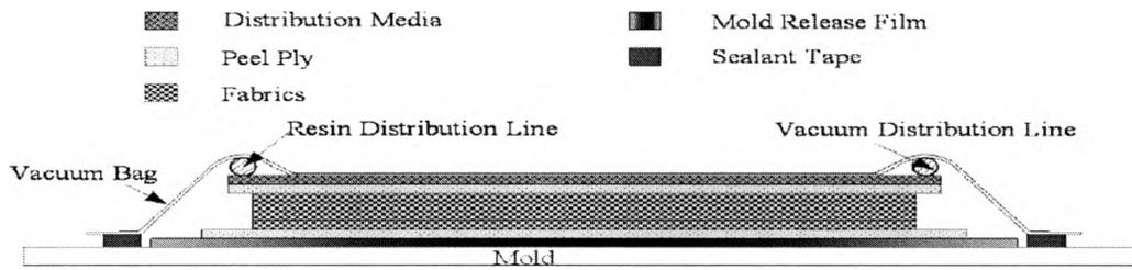
**Figure 2.6 Schematic for VARTM (Tate, 2004)**
