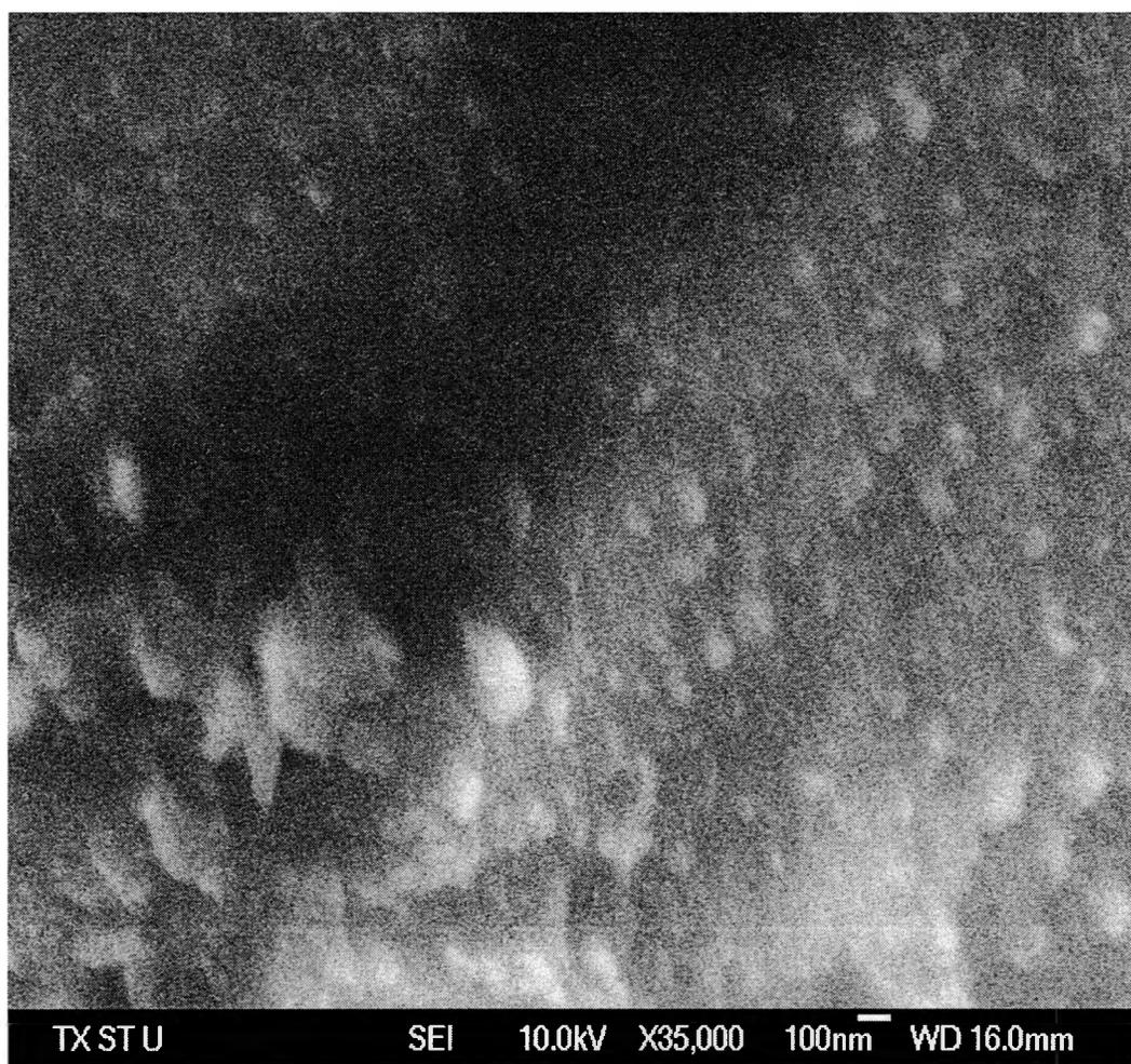
**Figure 2.15: Micrograph of Nanosilica in Epoxy**
