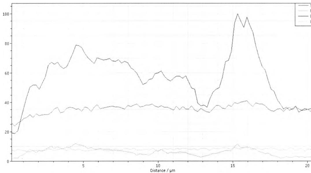
**Figure 2.16b: EDS showing material constituents of Nanosilica in Epoxy**
