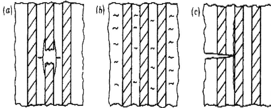
**Figure 1.8: Fatigue damage mechanisms in unidirectional composites under loading parallel to fibers: (a) fiber breakage, interfacial debonding; (b) matrix cracking; (c) interfacial shear failure (Talreja, 1987).**
