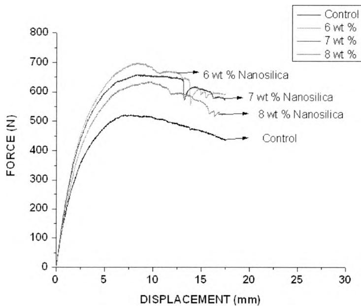
**Figure 4.5: Load vs displacement graph of control and nanocomposites**
