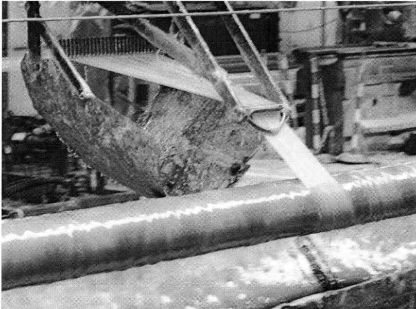
**Figure 2.4: Filament winding**
