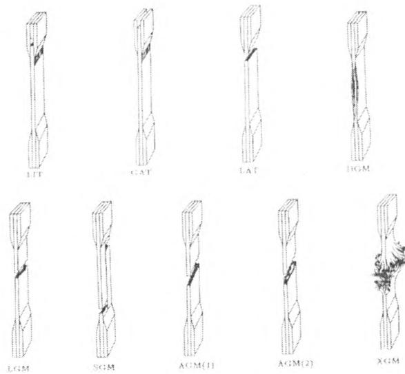
**Figure 3.4 Typical Tensile Test Failure Modes (ASTM D3039)**
