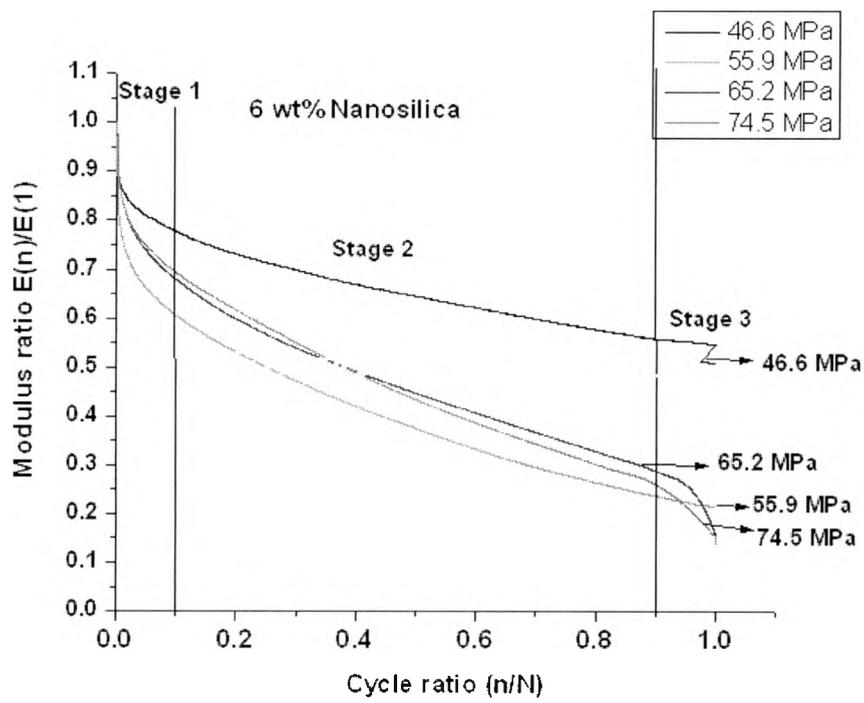
Figure 4.16: Stiffness degradation curve of nanomodified specimens
