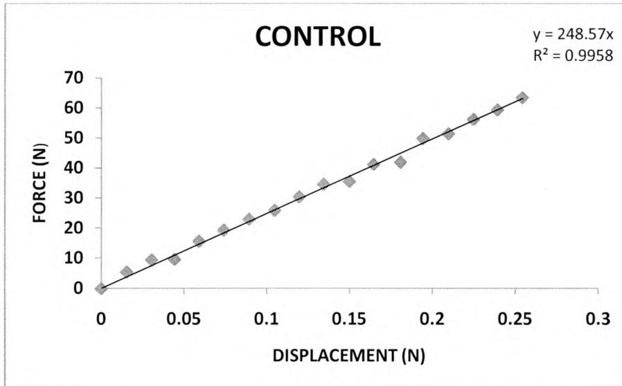
**Figure 4.6: Slope of initial linear portion for control composites**
