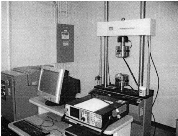
**Figure 3.1 MTS servo hydraulic test system**
