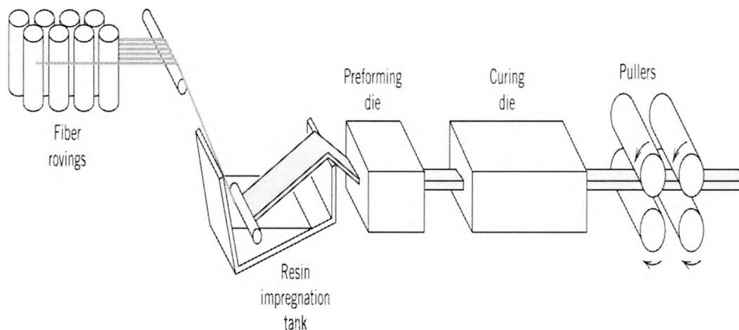
**Figure 2.3: Pultrusion process (Callister, 2008)**
