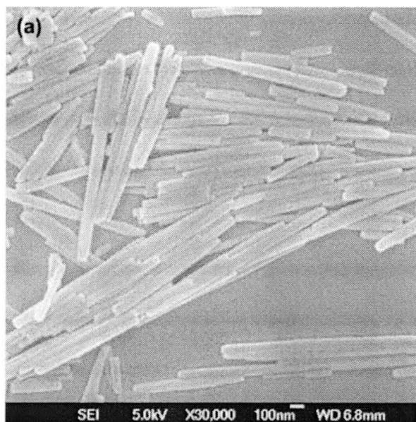
**Figure 1.3 Morphology of Halloysite Nanotubes (Yueping et al. 2007)**
