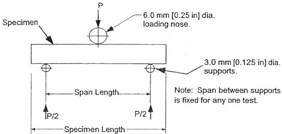
Where  $h$ =thickness, Specimen Length ( $L$ )=  $6h$ , Span Length ( $L_s$ )=  $4h$ , width ( $b$ )=  $2h$
