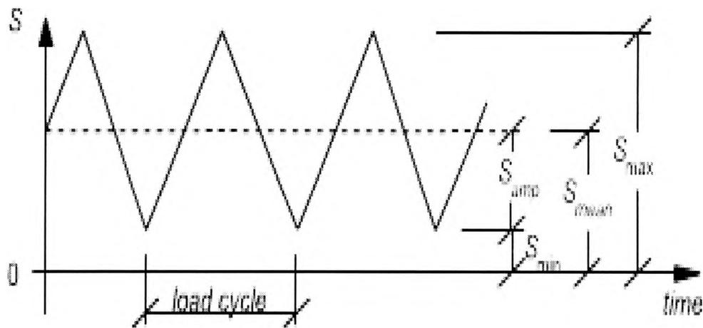
**Figure.1.4 Nomenclature for constant stress amplitude loading**
