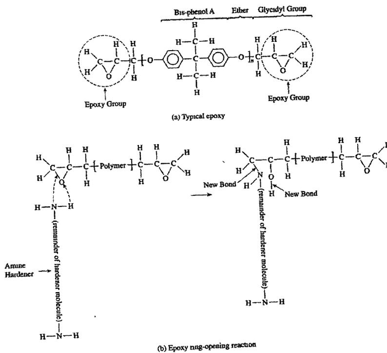
**Figure.1.2 Curing reaction of Epoxy**
