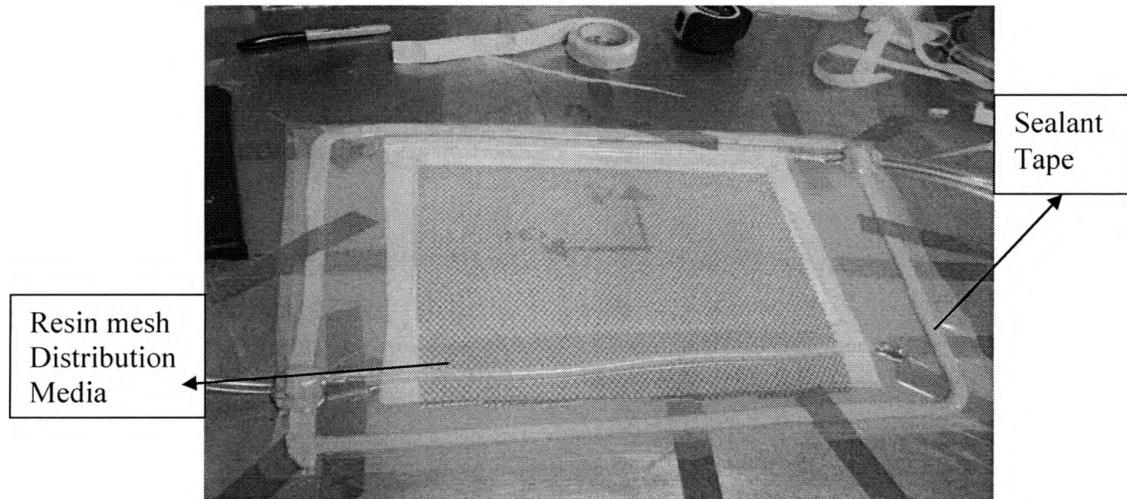
**Figure 2.12: Room Temperature VARTM Setup: Vacuum bagging**
