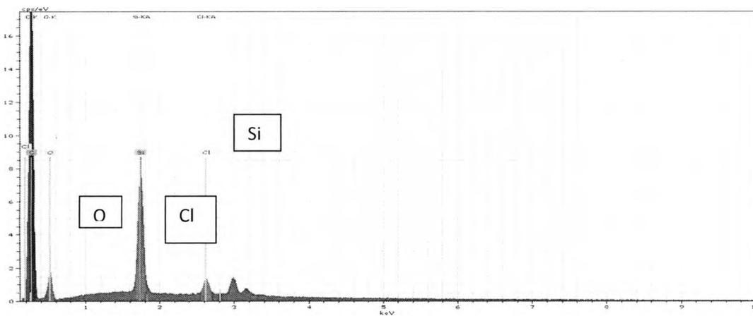
**Figure 2.16a: EDS showing material constituents of Nanosilica in Epoxy**
