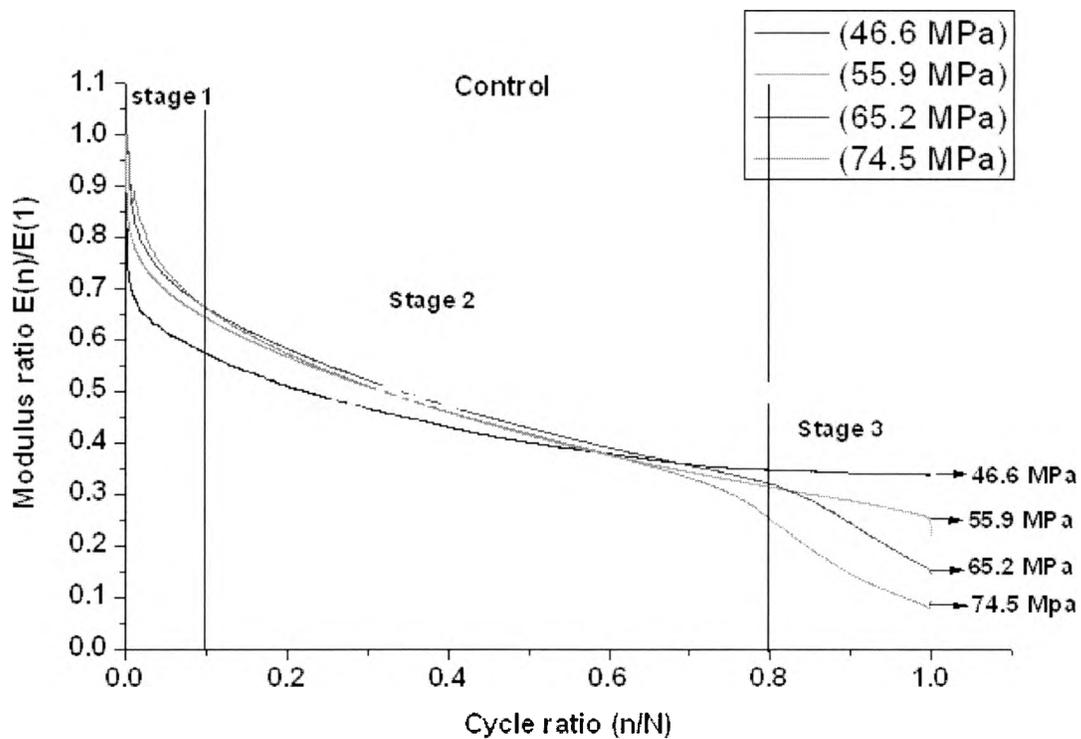
Figure 4.15: Stiffness degradation curve of Control specimens
