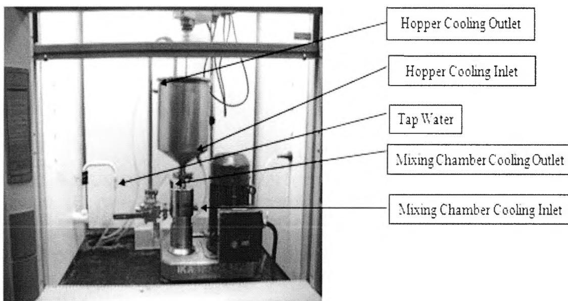
**Figure 2.7: IKA<sup>®</sup> Labor Pilot 2000/4 High Shear Mixer with cooling jacket (Tate, Kabakov, Koo, & Lao, 2009)**
