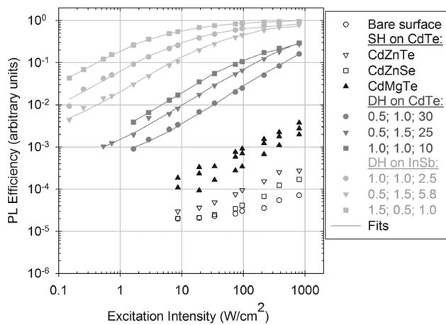
FIG. 2. The normalized PL dependence on excitation intensity shows the effect of single sided barriers (SH), two sided CdMgTe barriers (DH) on CdTe substrates, and DH growth on InSb substrates. The buffer layer thickness ( $\mu\text{m}$ ), the absorber layer thickness ( $\mu\text{m}$ ), and the resulting trap density ( $10^{10} \text{ cm}^{-2}$ ) are indicated for each DH. The measured PL signal was divided by the excitation intensity to obtain efficiency.
