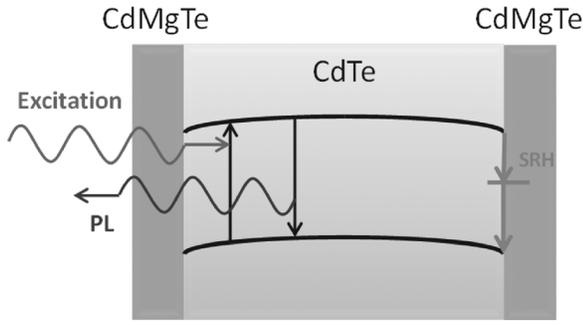
FIG. 1. Schematic of recombination in a CdMgTe/CdTe double heterostructure, consisting of an absorber layer between two barriers.
