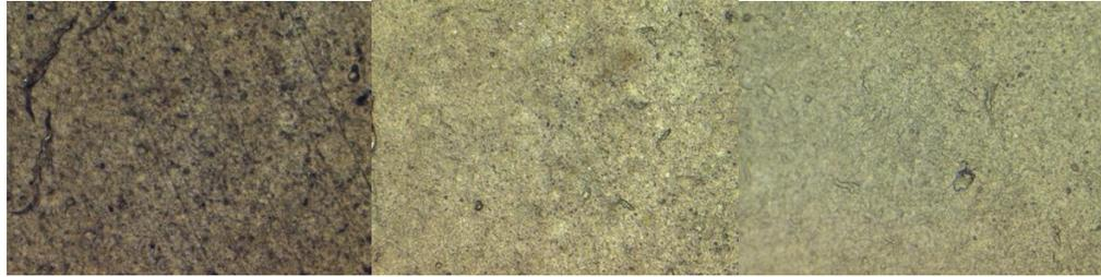
Figure 49: microscope imaging of PVOH 0.3 / MMT 0.45 at 24 layers at 5x, 10x and 20x resolution
