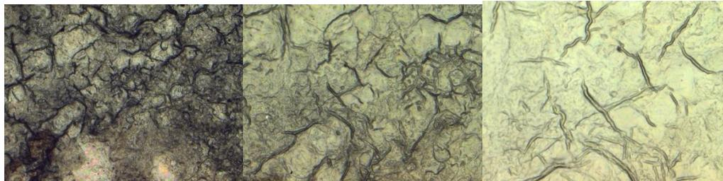
Figure 51: microscope imaging of PVP 0.3/LAP 0.45 at 24 layers 5x, 10x, 20x resolution
