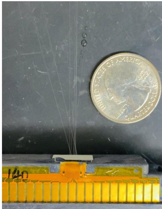
Figure 42: Dimatix print cartridge nozzle sizes as compared to a quarter
