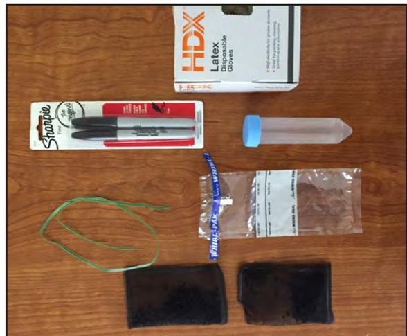
Figure 18. Materials Required for Sampling.
