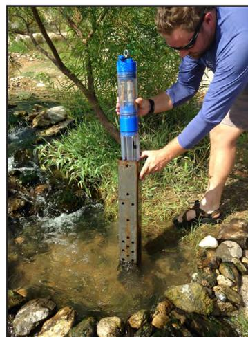
Figure 14. BSEACD Fluorimeter at PFSP Spring. Photo by Brian Hunt.
