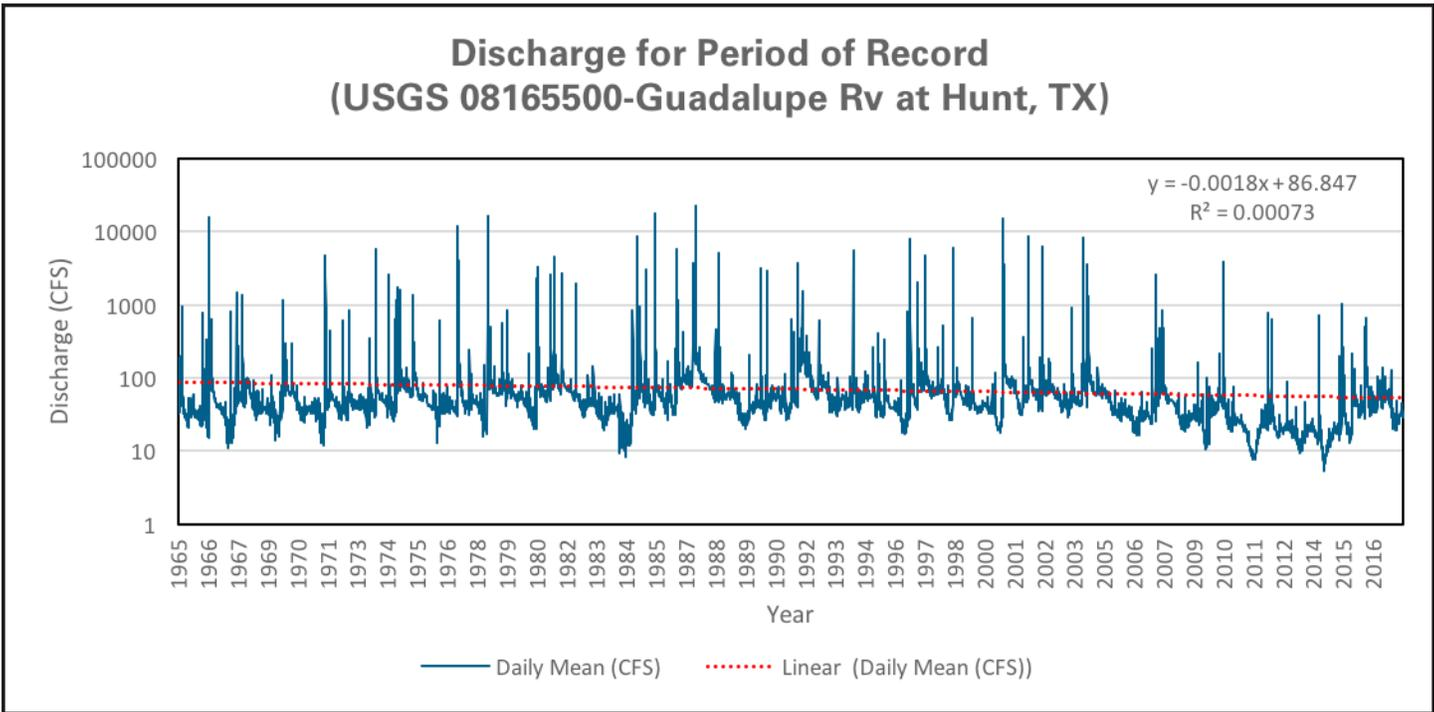
Figure 8 USGS Gaging Station 08165500 at Hunt, TX (1965-2017)
