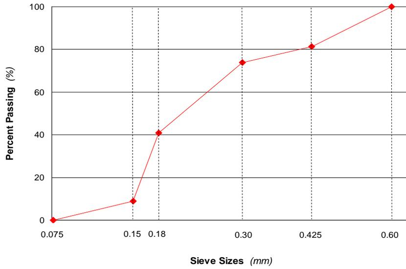
Figure 2. Gradation of CRM used in this study
