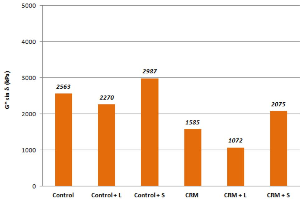
Figure 16.  $G^* \sin \delta$  of the binders with wax additives
