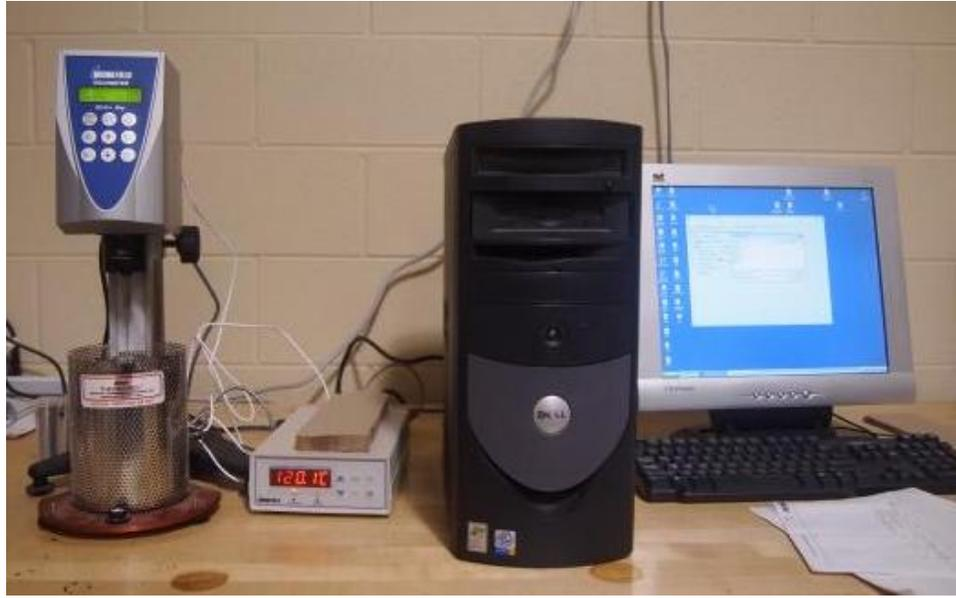
Figure 7. Rotational viscometer
