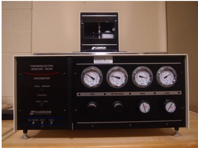
Figure 9. Bending Beam Rheometer (BBR)
