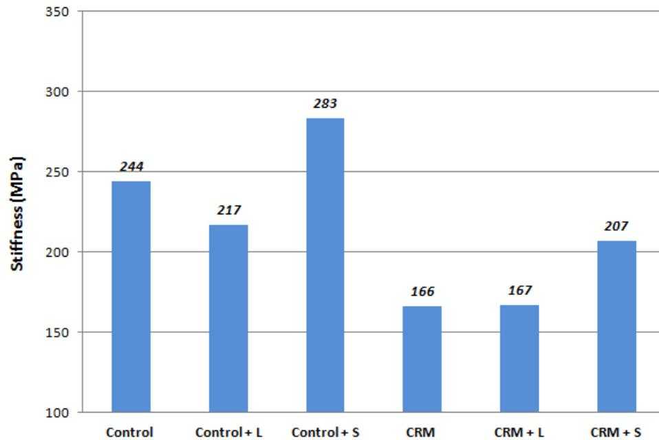
Figure 18. Stiffness at -12°C (after RTFO)
