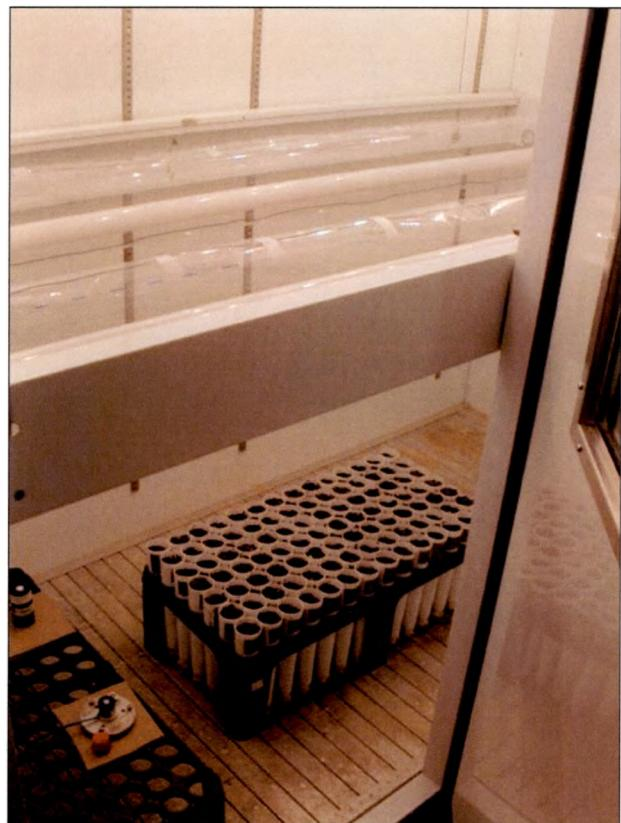
Figure 1. Growth chamber experimental set-up showing pot arrangement, sensor equipment positioning, and UV bulb set-up.
