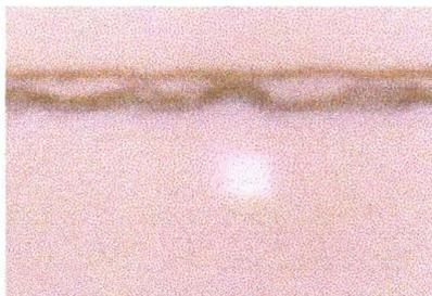
**Figure 3-20 Developed line and beam size for 5.8 mJ exposure**
