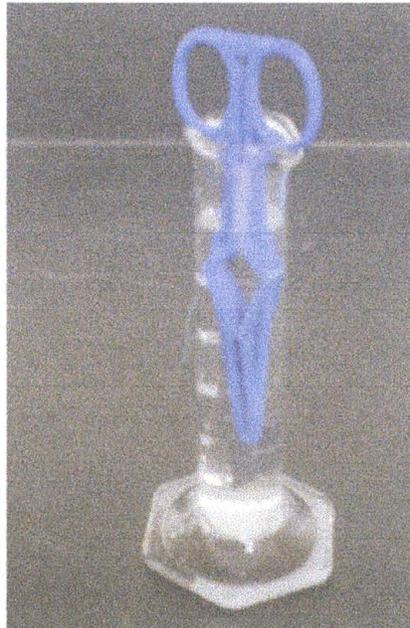
Figure C-1 A sample suspended in etchant.
