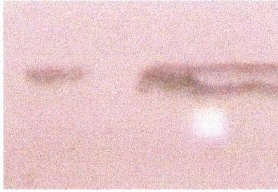
**Figure 3-21 Developed line and beam size for 2.3 mJ exposure**
