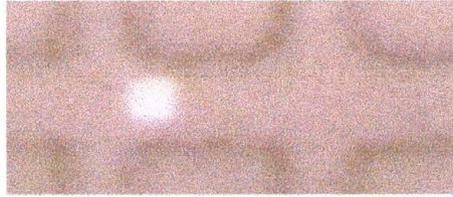
**Figure 3-14 Spot projected on larger sized photoresist pattern**
