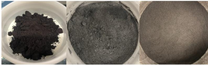
**Figure 14.** 50wt% NdFeB/PA12 at zero, two and five mixing cycles of three minutes.
