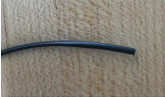
**Figure 16.** Die swell in NdFeB/PA12 filament.
