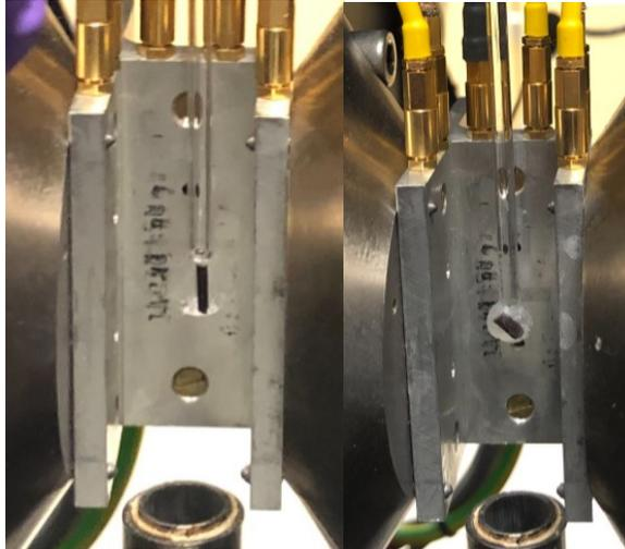
**Figure 26.** Samples on the rod holder. Left, correct position. Right, misaligned position.
