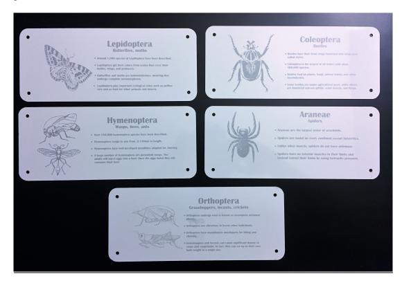
The above signs were made in the Bobcat Made Makerspace on the Texas State Campus. To begin, the sign blanks were ordered from amazon.com. They are roughly 10.25 x 4.25". These dimensions were used to create the layout and design, which was completed with Adobe Acrobat. Once each sign had been designed and formatted correctly, the files were saved to a zip drive and taken to the Makerspace where they were sent directly to the laser etching and engraving machine. There was a fair amount
