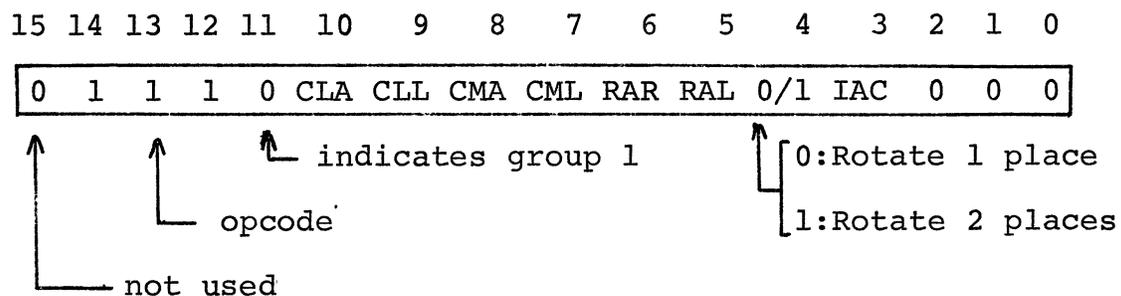
It is seen from this diagram that the entire word is used to specify which operation is to be performed. This is possible since no operand is required for these instructions. Bits 5-10 and bit 3 specify the operation indicated below.
