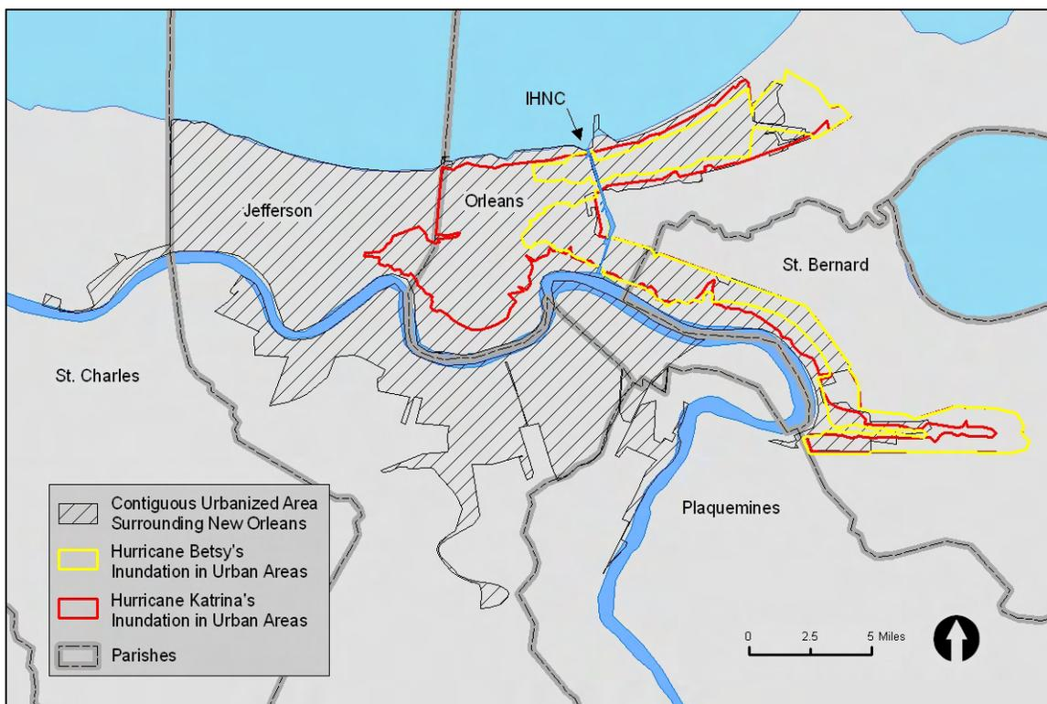
**Figure 5: Generalized Patterns of Inundation Produced by Hurricanes Betsy and Katrina in Urban Areas. Note the IHNC. Floodwall failures along this canal accounted for much of the flooding during both storms.**
