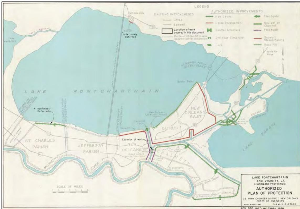
**Figure 10: Levee Improvements Authorized by Lake Pontchartrain and Vicinity, Louisiana, Hurricane Protection Project (United States Army Corps of Engineers 1965). These improvements, though not yet fully implemented as of this writing, structurally and symbolically represent the contemporary hurricane protection system.**
