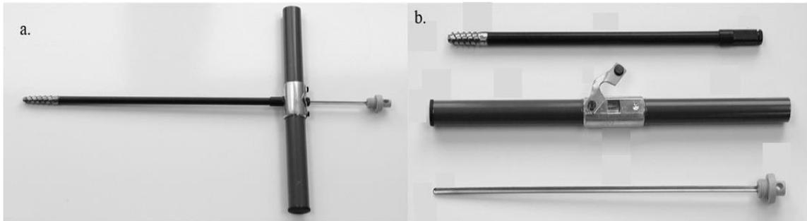
Figure 7. The increment borer showing: a.) the equipment assembled; b.) the equipment disassembled (Grissino-Meyer, 2003).
