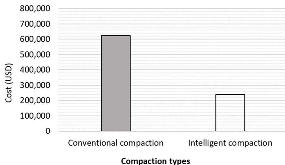
Figure 1. Roadway lifecycle cost of conventional and intelligent compaction.
