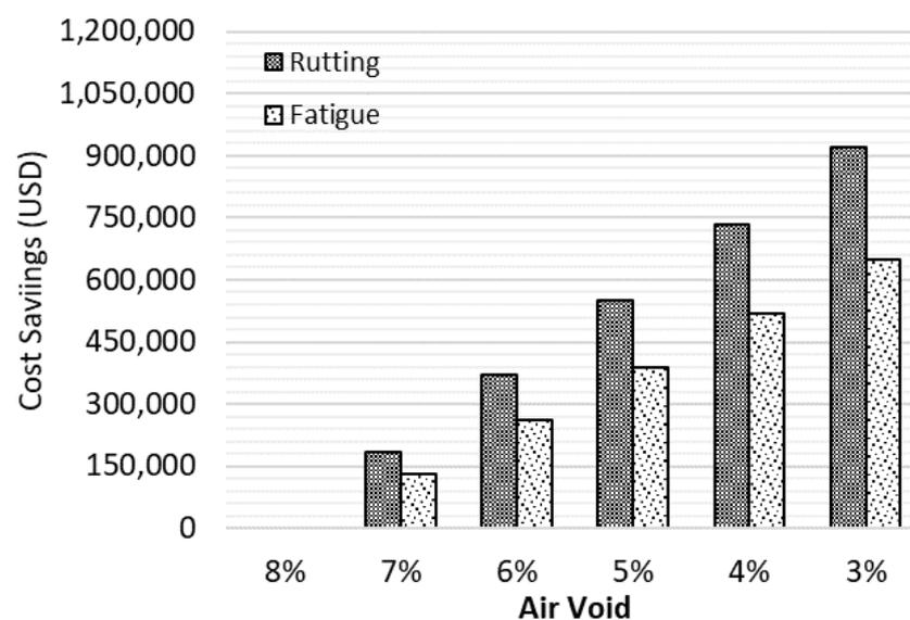
**Figure 3.** Cost savings with IC due to rutting and fatigue improvement.
