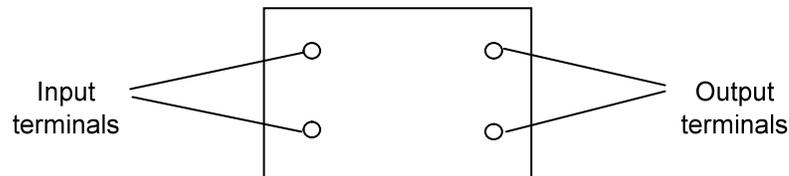
**Figure 2.2.3: Top view of SSR**
