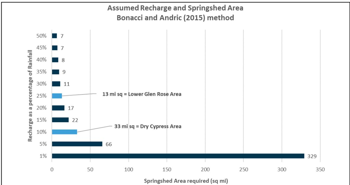
**Figure 9.** Results of assumed recharge as a percentage of precipitation and the calculated springshed area. The area of Dry Cypress Creek watershed is about 31 square miles, or about 10 percent of precipitation. The Lower Glen Rose has an area within Dry Cypress Creek watershed of 12.1 square miles, or about 25 percent of precipitation.
