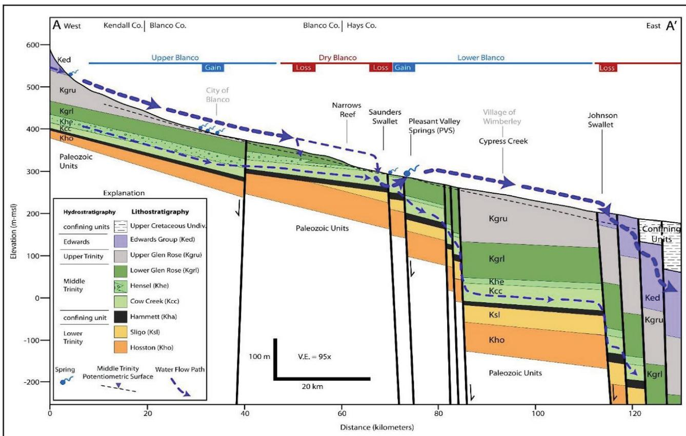
**Figure 16.** Conceptual cross section of the entire Blanco River showing surface-water/groundwater interaction (from Smith and others, 2015). (co. = county, km = kilometers, m = meters, m-msl = meters above mean sea level, undiv. = undivided, V.E. = vertical exaggeration)
