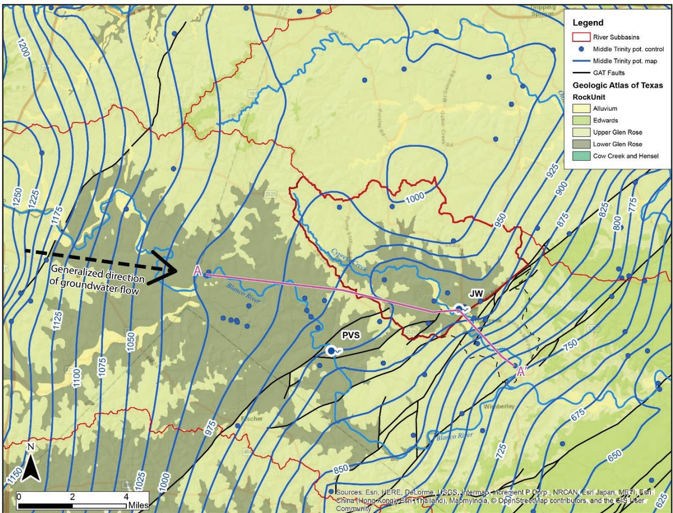
**Figure 7.** Regional potentiometric (water level) surface of the Middle Trinity Aquifer in March 2018. Elevations in feet above mean sea level. Data from Hunt and others (2019). Cross Section A to A' shown in Figure 6.
