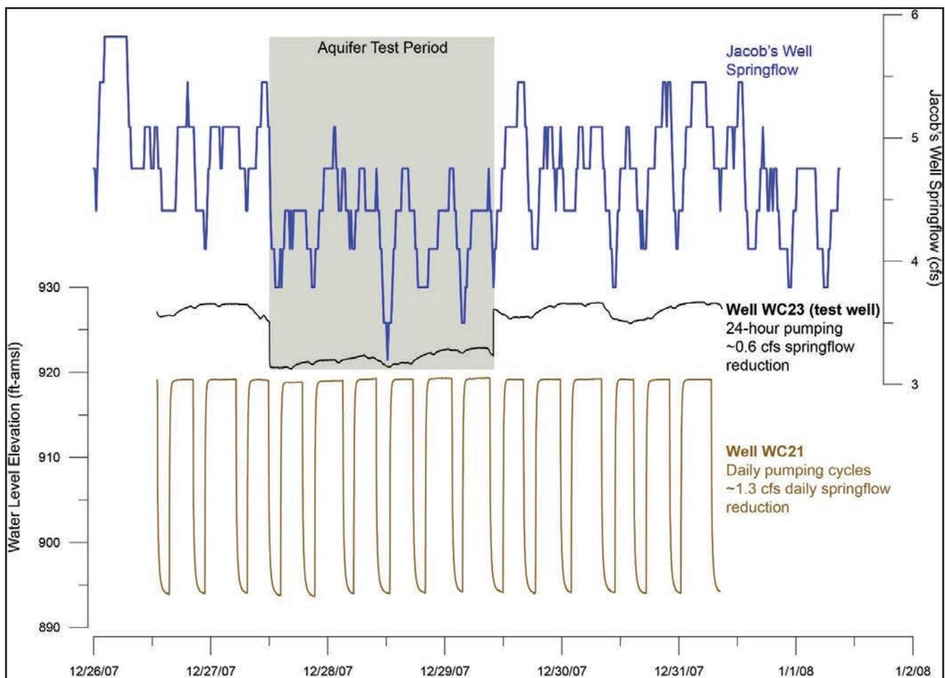
**Figure 12.** Hydrograph of the WC23 pump test with the test period shaded. Both wells WC21 and WC23 show an influence on the flows at Jacob's Well. Location of wells shown on Figure 13. (cfs = cubic feet per second, ft-amsl = feet above mean sea level)
