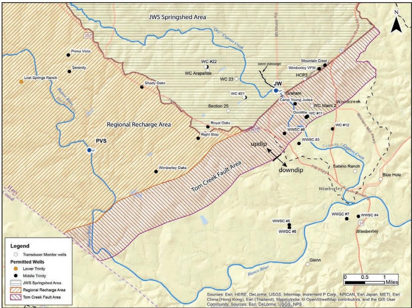
**Figure 13.** Location of transducer (monitor) and public water system wells in the study area. Note the up-dip area corresponds to wells located within the Tom Creek Fault Area and Jacob’s Well Springshed areas. (JW = Jacob’s Well Spring)
