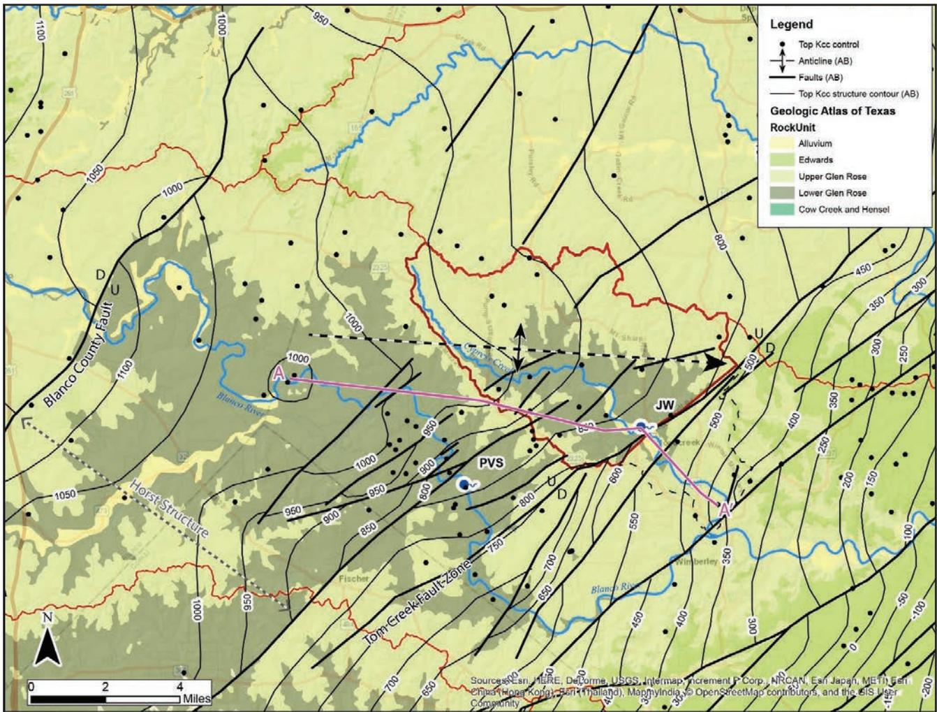
**Figure 5.** Structure contour map of the top of the Cow Creek (contours in feet above mean sea level). Contours, control, and faults from Al Broun (unpublished data). Figure modified from Wierman and others, 2010. Cross section A to A' is shown in Figure 6.
