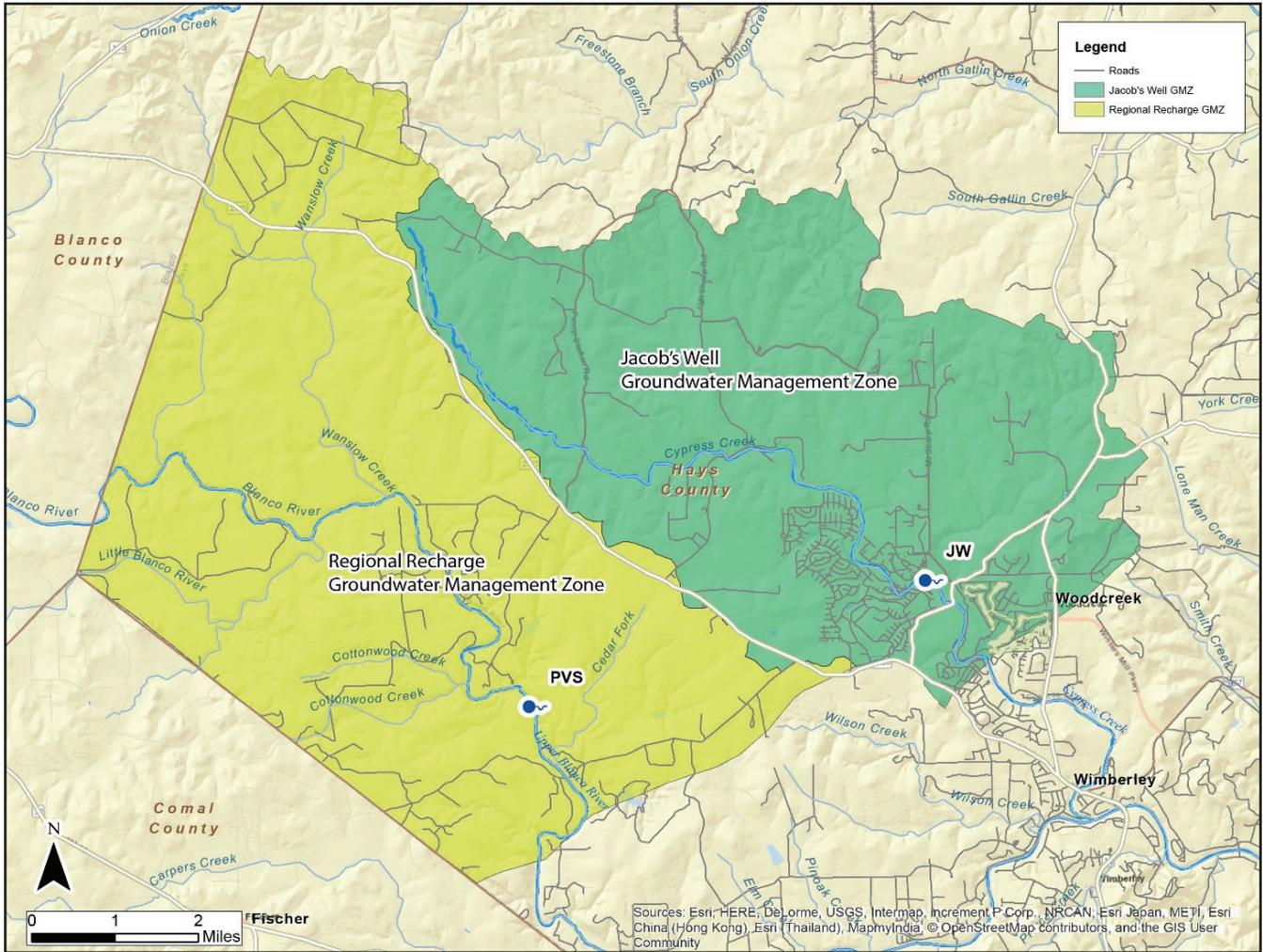
**Figure ES-1.** Areas of hydrologic influence to Jacob’s Well shown in hatched areas. Potential groundwater management zones are shaded green and yellow. The area of the Jacob’s Well Groundwater Management Zone is 34 square miles and the area of the Regional Recharge Groundwater Management Zone is 56 square miles.
