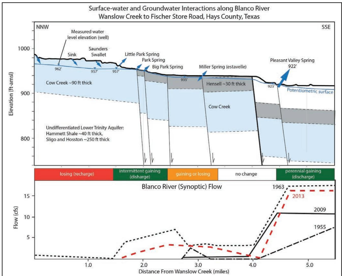
**Figure 17.** Detailed cross section and flow rate graph show the surface-water/groundwater interaction of the spring reach of the Blanco River from Gary and others, (2013). Synoptic Blanco River flows indicates flows that occurred within a short period of time, generally less than a few weeks. Synoptic flow events were made during low-flow conditions.
