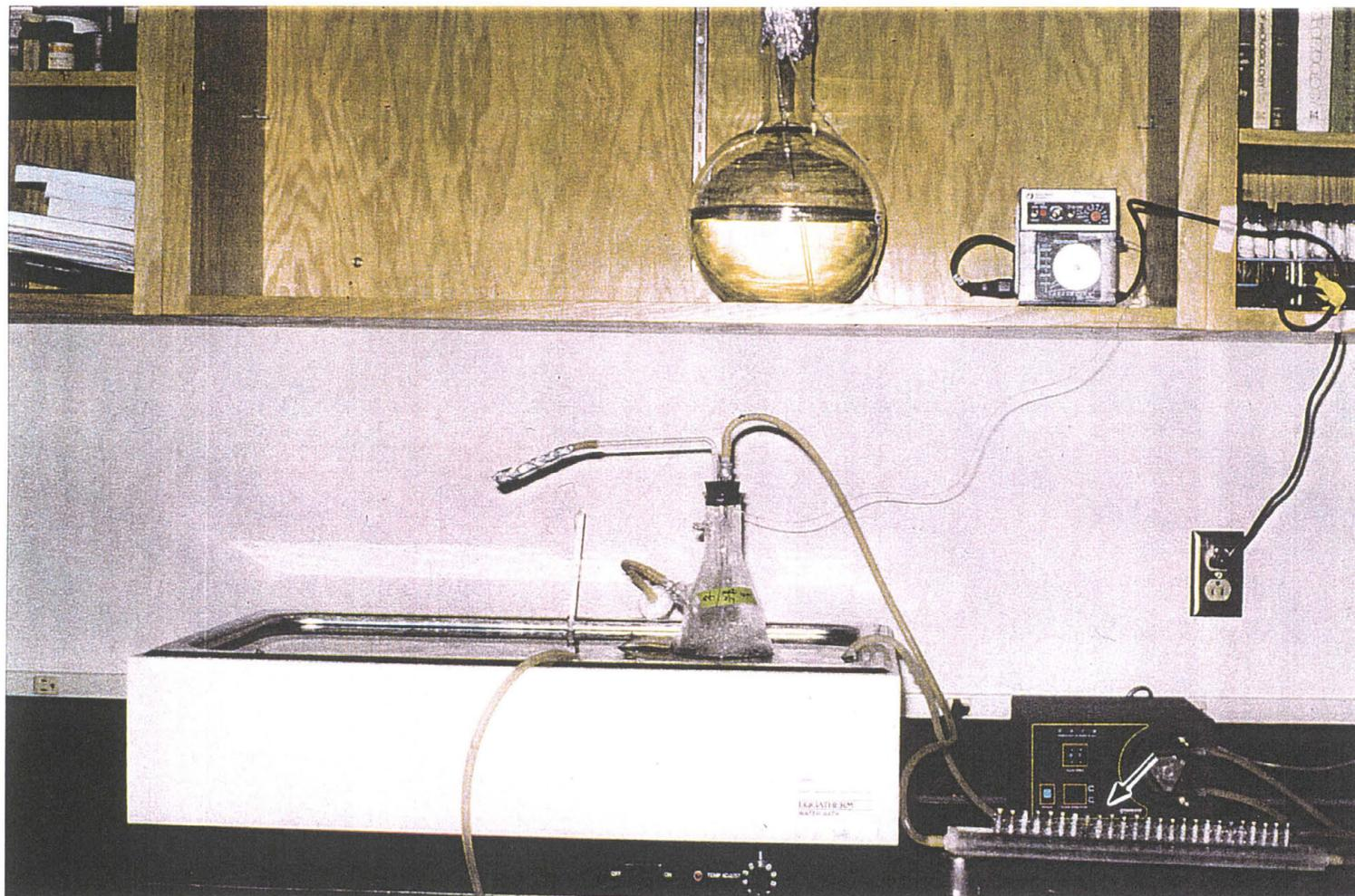
Fig. 1 Photograph of experimental apparatus including: fresh media flowing through pump to chemostat, chemostat in 37°C water bath, aeration from the rear, waste flowing to receptacle below, and Modified Robbins Device connected by peristaltic pump marked with an arrow.
