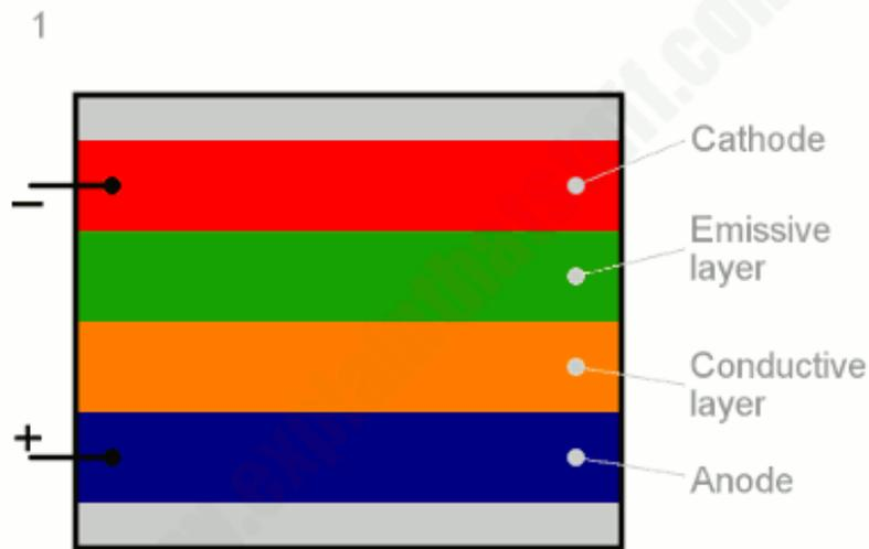
Figure 4. Standard OLED system. <sup>15</sup>
