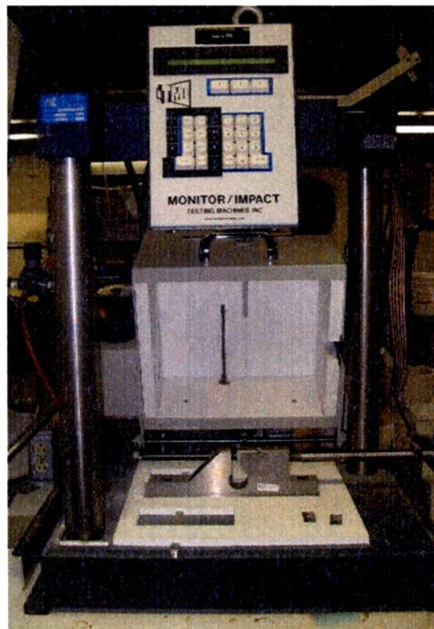
Figure 34: Impact testing machine
