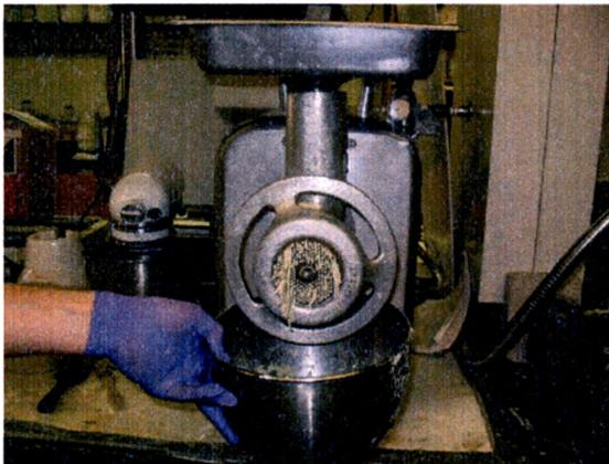
Figure 24: Hobert Commercial Auger Extruder (model 4822)
