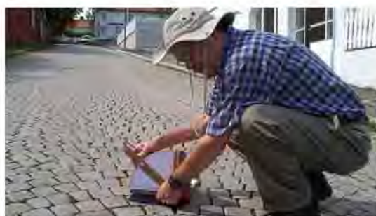
Roger Sinnott uses shadows cast by the sun to measure the slope of Havnegata, the road between the Grand Hotel and the Kiøsterud estate in Åsgårdstrand as part of a topographic survey of the town. (photograph Ava Pope)
