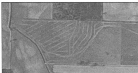
*Figure 2. Example of herringbone and parallel tile placement, Allen County, Ohio, late October, 1956.*
