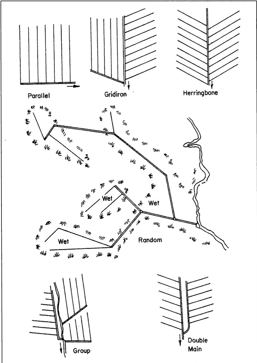
Figure 1. Common drainage tile patterns.
