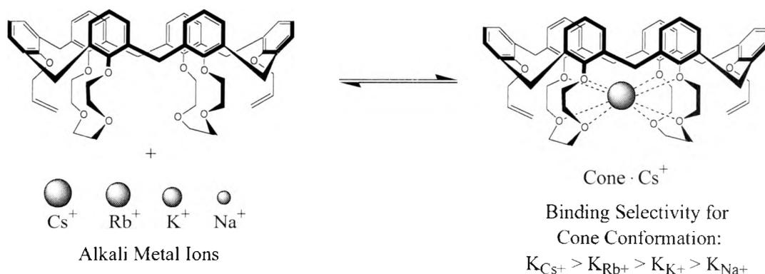
**Figure 1.10** Metal binding study for bis-bridged calix[6]arene crowns.
