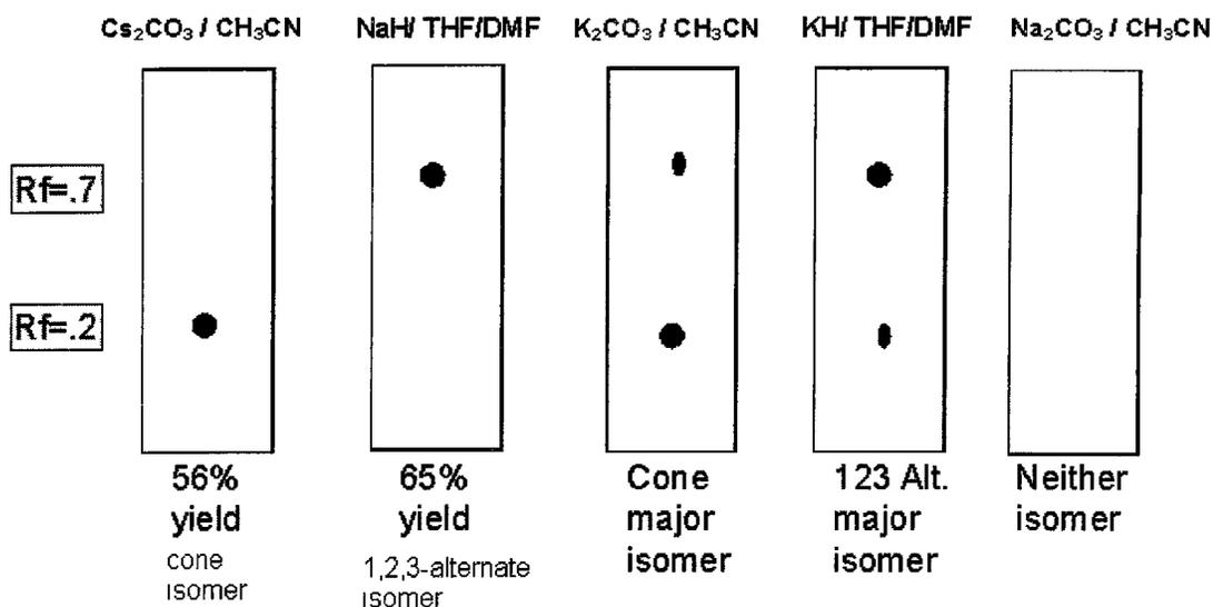
**Figure 3.4** The TLC results from varied base and solvent conditions.
