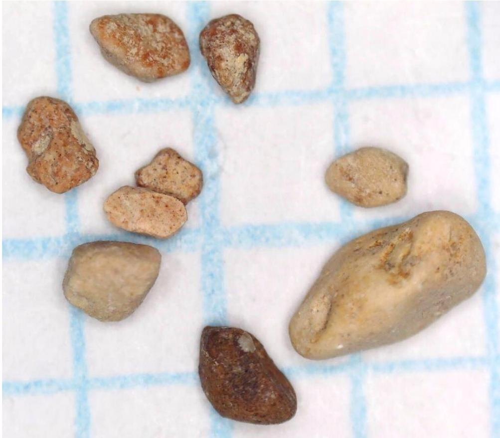
Figure 8-27. Examples of rounded gravel observed in FN 60299. Unit C1 L6, at approximately 57x magnification; 1 Cell = 2.5 mm (0.1 in). Note the varied lithic materials and size range within the 1-2mm fraction.
