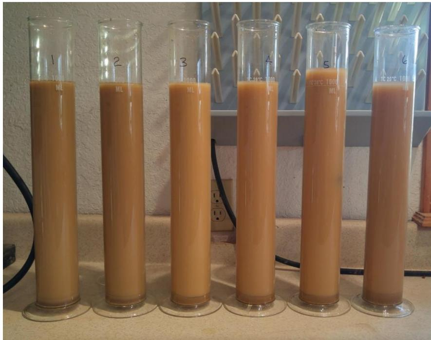
Figure 5-6. Fine-fraction sediment samples settling in graduated cylinders during hydrometer-based particle size analysis.
