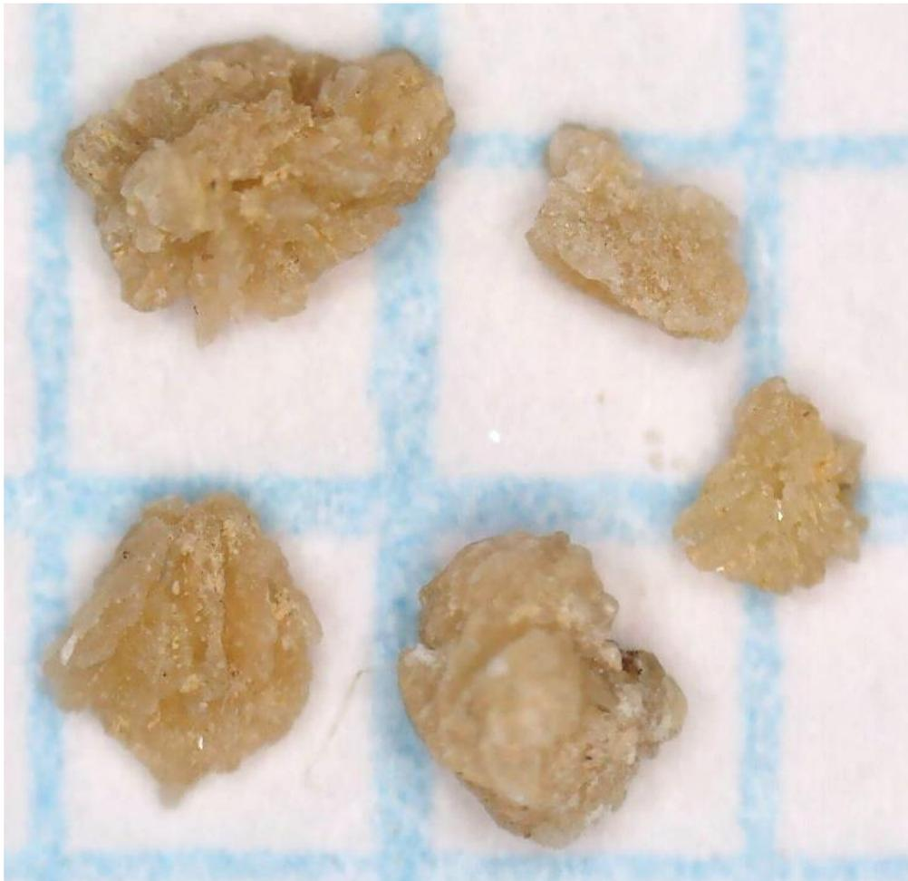
Figure 8-28. Crystalline gypsum fragments observed in FN60092. Unit C2 L1, at approximately 57x magnification; 1 Cell = 2.5 mm (0.1 in)
