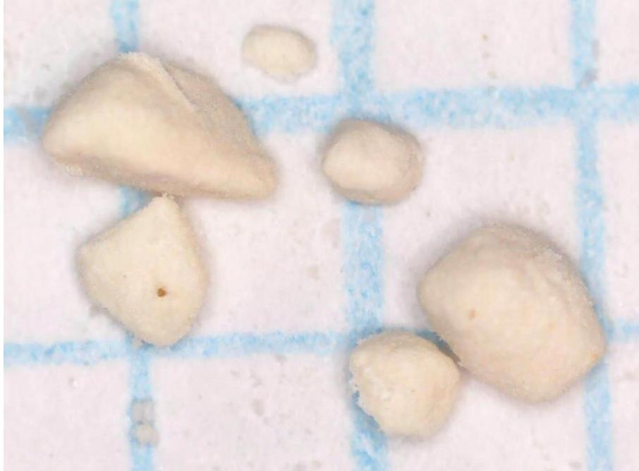
Figure 8-29. Rounded gypsum nodules observed in FN60092. Unit C2 L1, 1 Cell = 2.5 mm (0.1 in)
