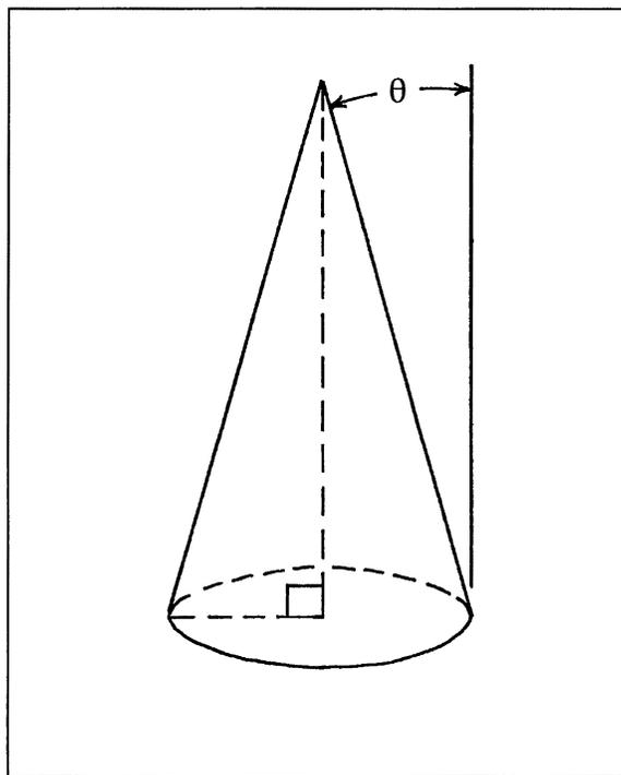
Figure 17. Measurement of taper for a right circular cone.
