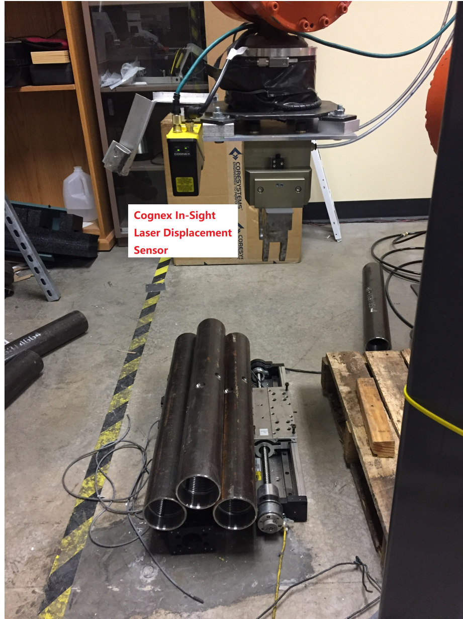
Figure II.6: Cognex Laser Displacement Sensor with Robot Gripper.
