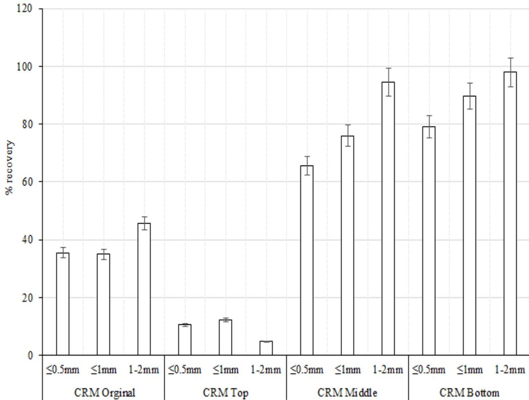
Figure.7 % recovery at 64°C of effective particle size of crumb rubber at 0.1 kPa
