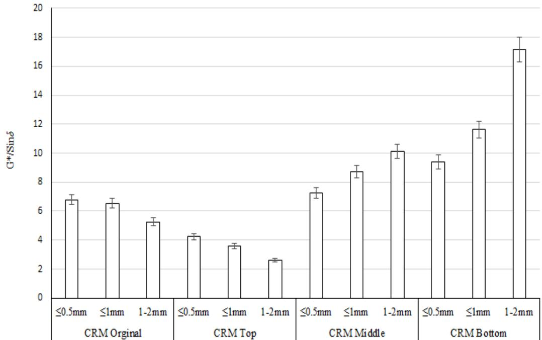
Figure.5 Viscoelasticity( $G^*/\sin \delta$ ) at 64°C of effective particle size of crumb rubber for original sample and top, middle, bottom part(Conditioned)
