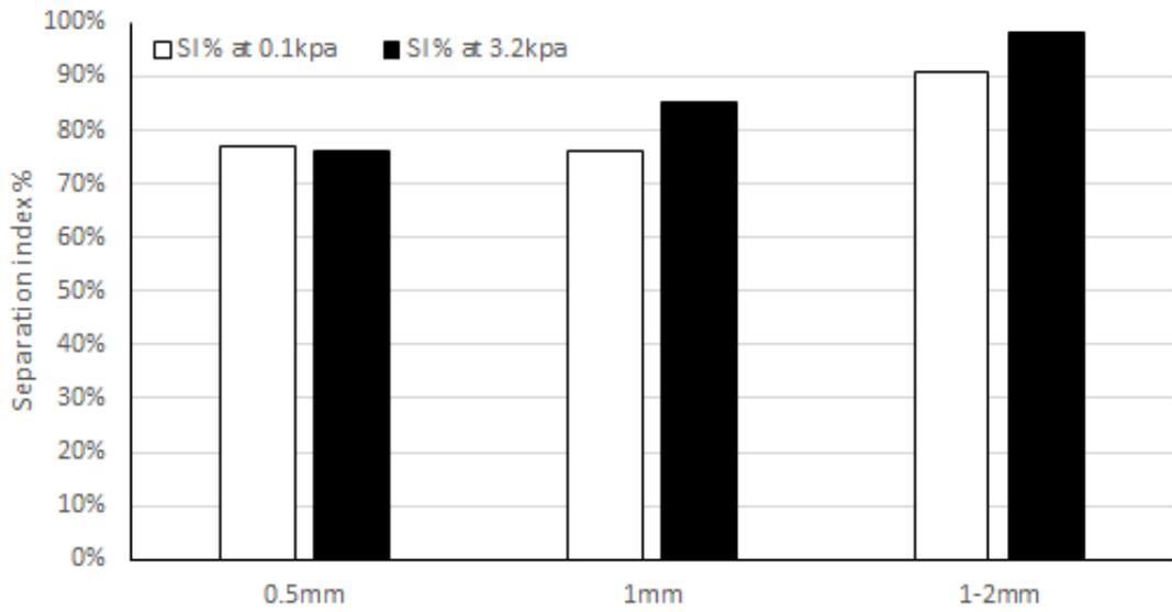
Figure.9 Separation Index % at 64°C of effective particle size of crumb rubber for 0.1 kPa and 3.2 kPa
