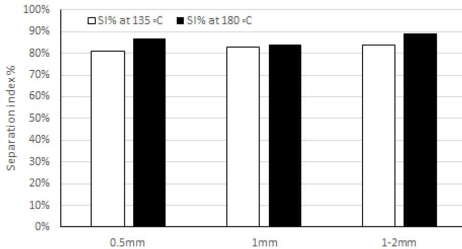
Figure.4 Separation index % for viscosity for effective particle size at 135°C and 180°C considering only top and bottom part (Conditioned)
