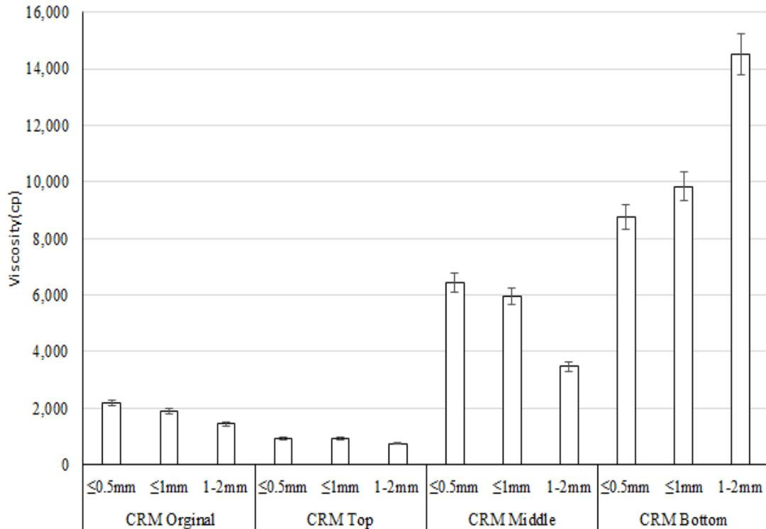
Figure.2 Viscosity at 135°C of effective particle size of crumb rubber for original sample and top, middle, bottom part (Conditioned)
