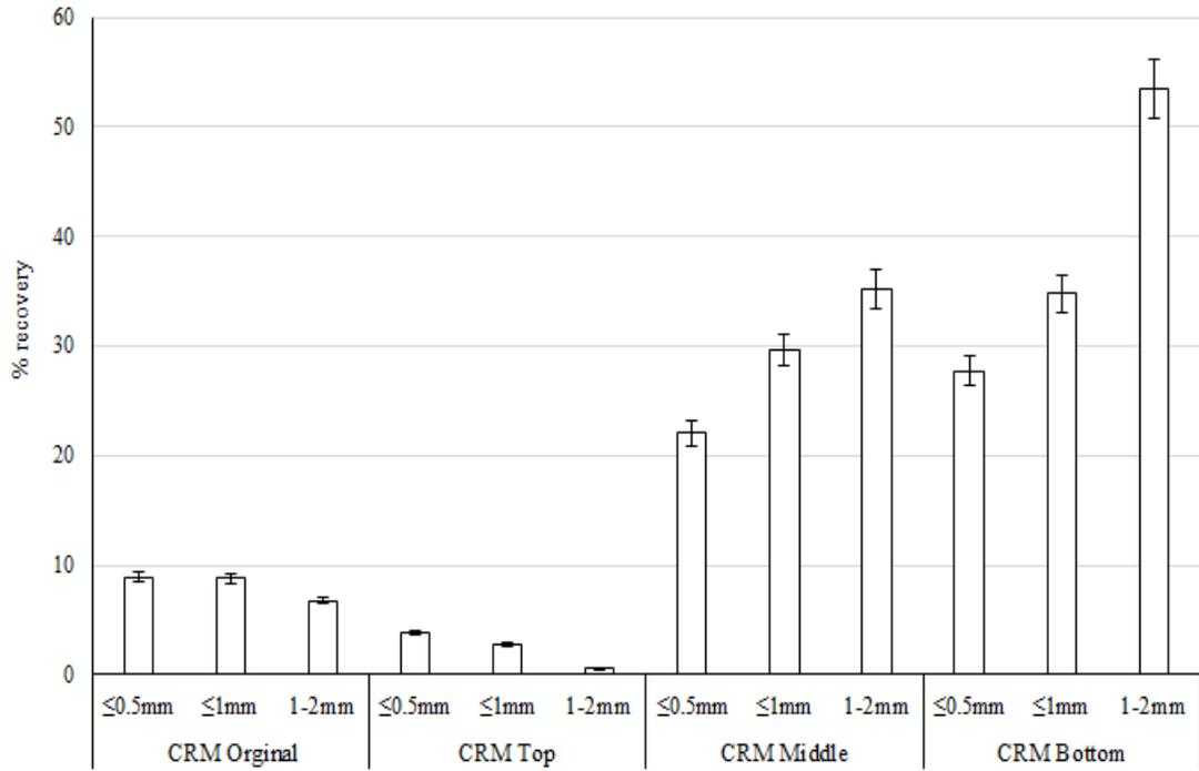
Figure.8 % recovery at 64°C of effective particle size of crumb rubber at 3.2 kPa
