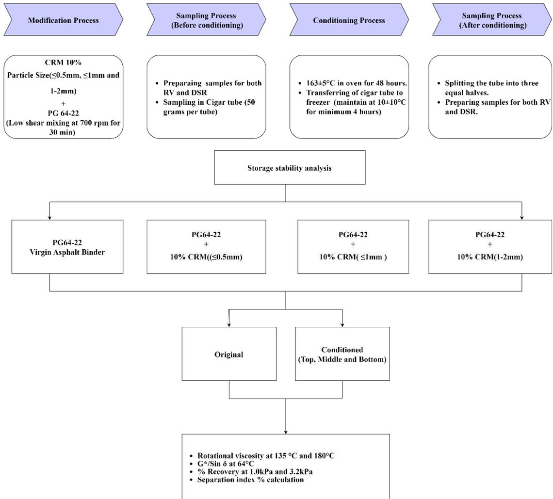
Figure.1 Experimental design model
