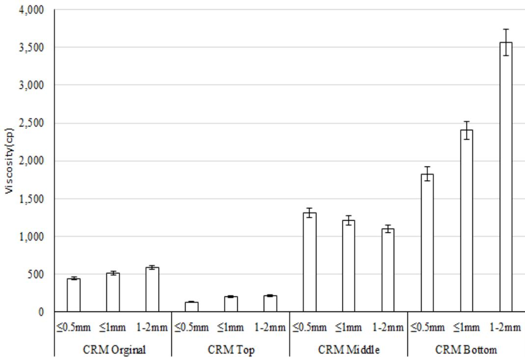
Figure.3 Viscosity at 180°C of effective particle size of crumb rubber for original sample and top, middle, bottom part (Conditioned)
