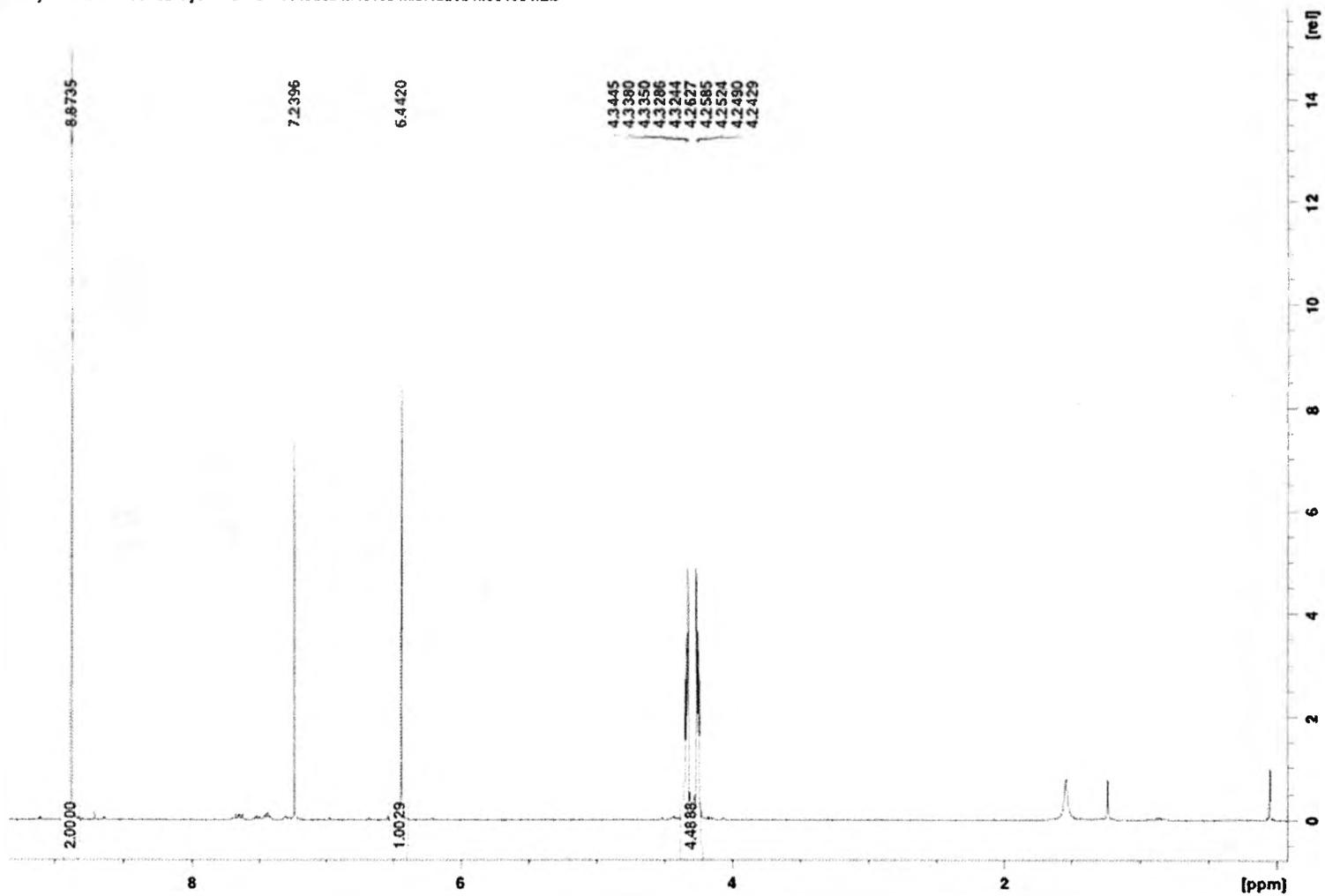
Spectrum 24: 2-Chloro-5-(3,4-ethylenedioxythiophen-2-yl)-pyrimidine  $^1\text{H}$  NMR in  $\text{CDCl}_3$
