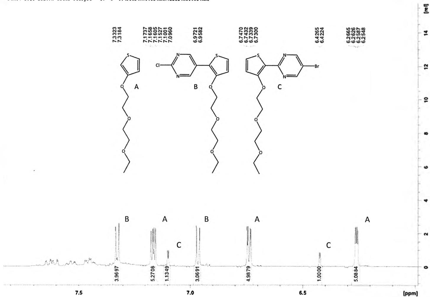
Spectrum 15: B3ETPM reaction mixture thiophene region  $^1\text{H}$  NMR in  $\text{CD}_2\text{Cl}_2$
