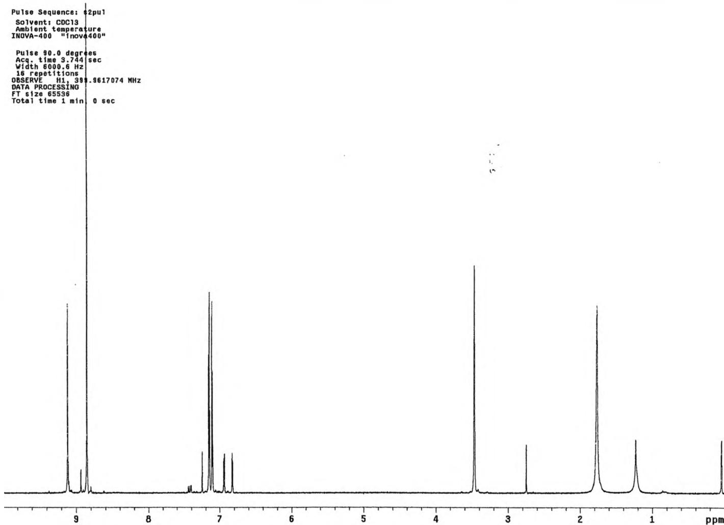
Spectrum 16: 5-Bromo-(2-pyrimidin-5-yl)-thiophene <sup>1</sup>H NMR in CDCl<sub>3</sub>
