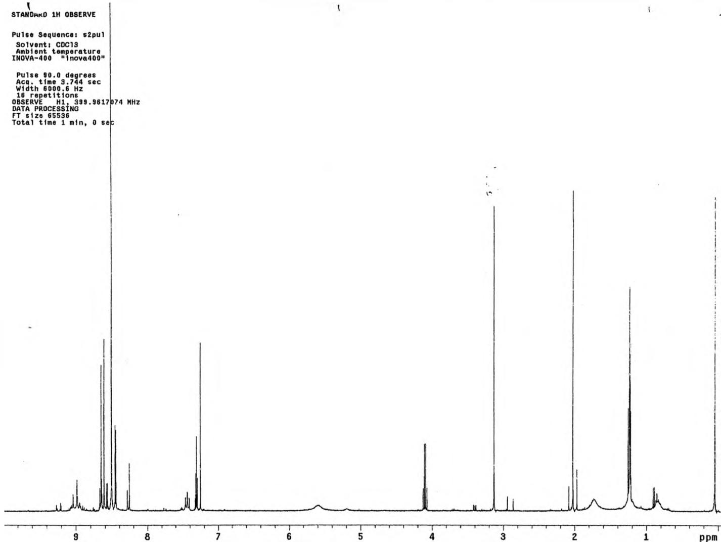
Spectrum 20: Ullmann coupling of 5-bromo-2-iodopyrimidine <sup>1</sup>H NMR in CDCl<sub>3</sub>
