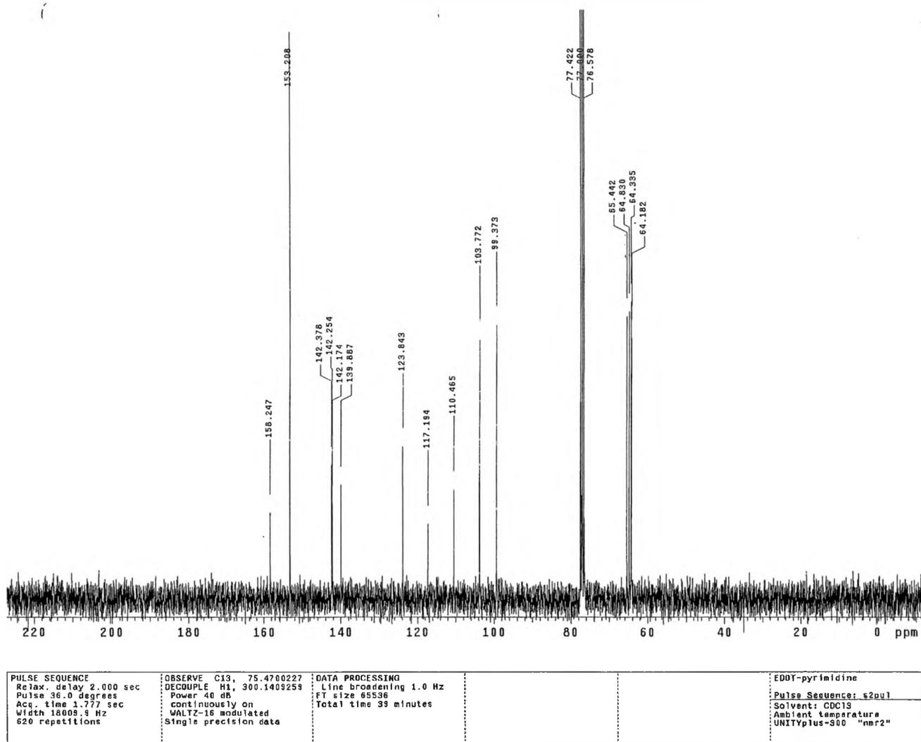
Spectrum 13: BEPm  $^{13}\text{C}$  NMR in  $\text{CDCl}_3$
