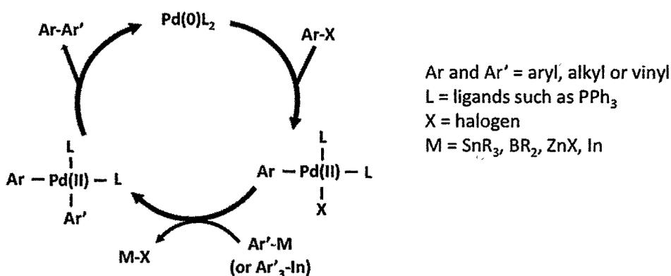
**Figure 6:** General palladium (0) catalyzed mechanism for carbon-carbon bond formation
