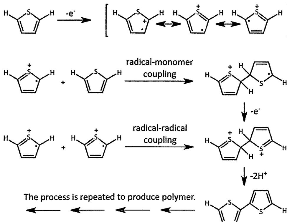
**Figure 7:** Oxidative polymerization of thiophene<sup>5</sup>
