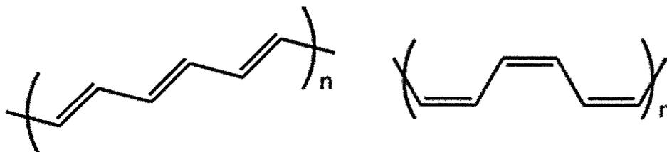
**Figure 1:** Structures of *trans*-polyacetylene (left) and *cis*-polyacetylene (right)
