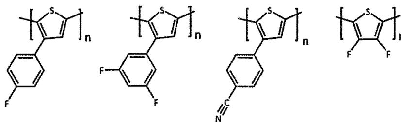
**Figure 4:** Polymers with pendant electron withdrawing groups<sup>21,22</sup>
