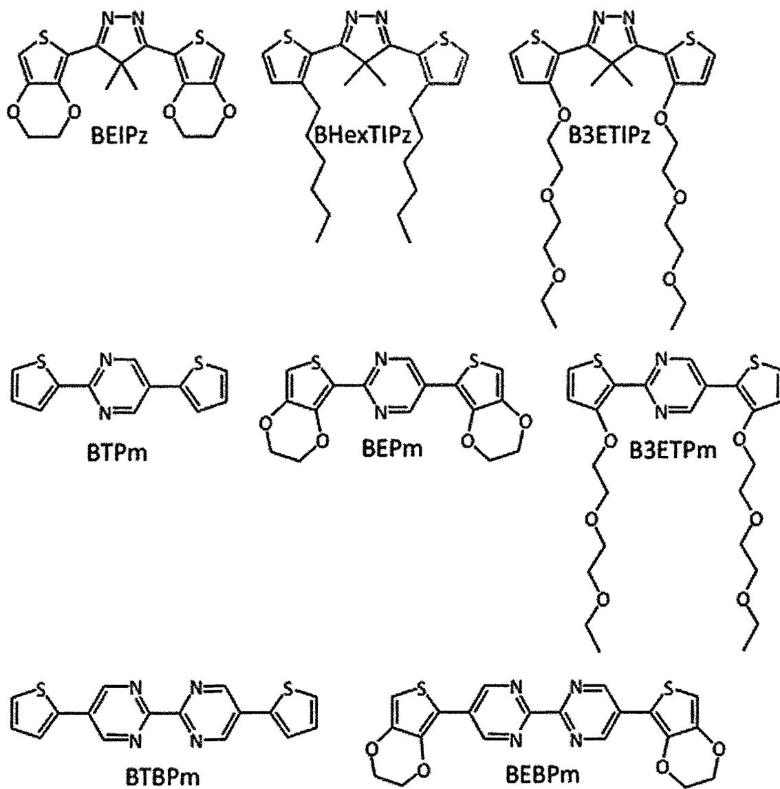
**Figure 9:** Proposed monomers to be used to synthesize n-doping polymers
