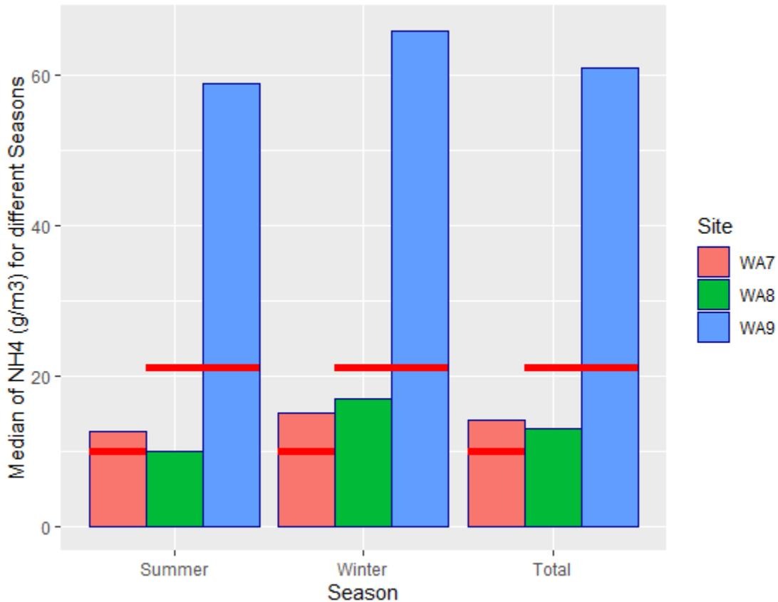
Figure 4.12: Ammonium for a Different Season. The red lines represent the ANZECC trigger value for NH<sub>4</sub>
