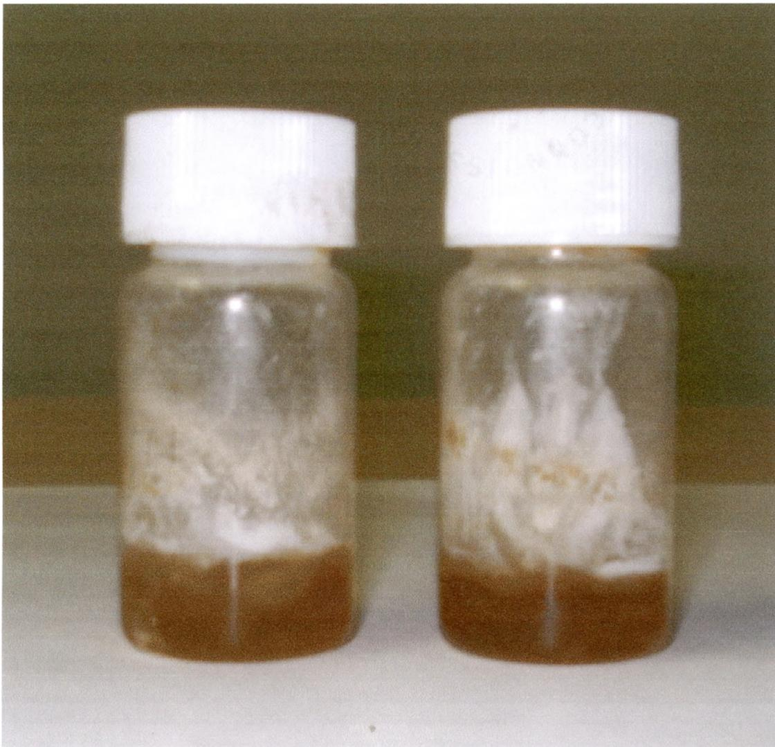
**Figure 9. Incomplete Nanoclay Polymerization.** Notice the excess crystallized lactide with clay trapped inside along the walls of the vials.
