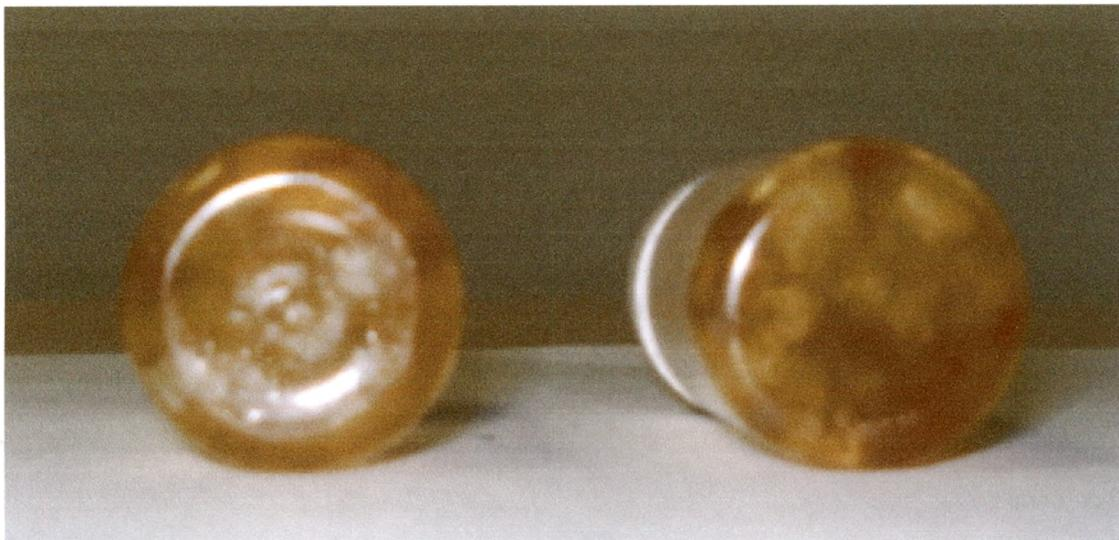
**Figure 10. Heterogeneous Clay-Polymer Mixture.** Notice the darker clay regions.
