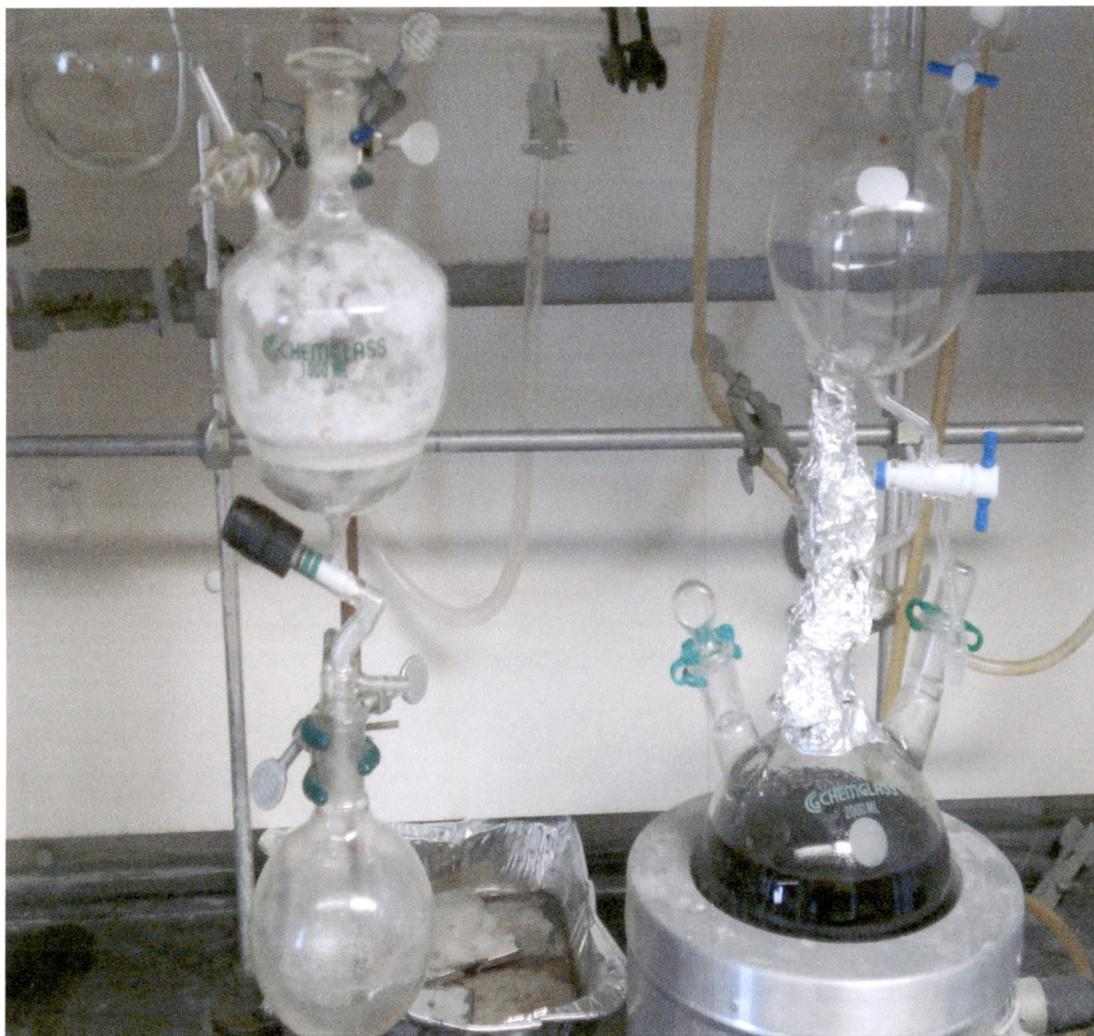
**Figure 5. Air-Free Filter Flask (left) and Toluene Still (right).**
