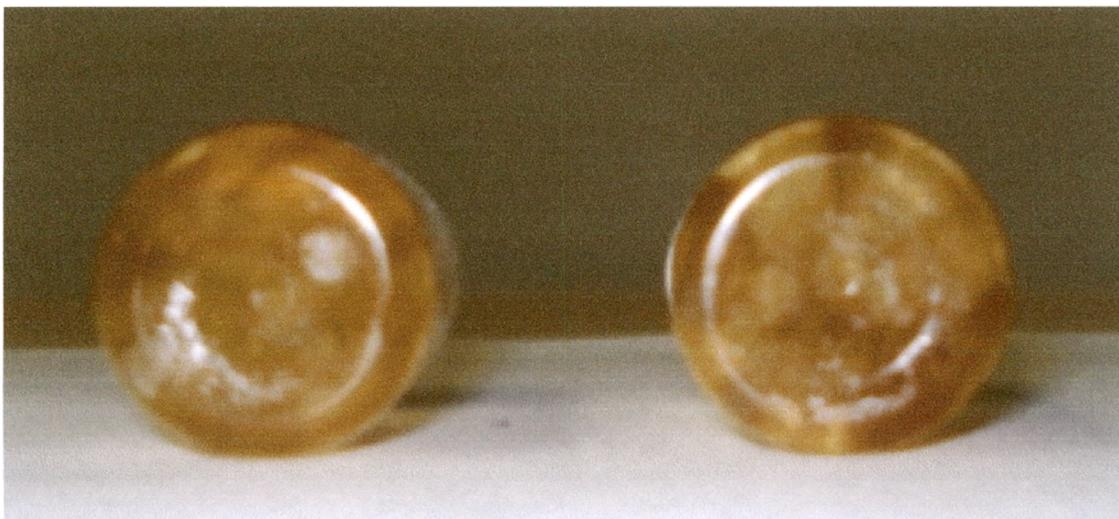
**Figure 11. Heterogeneous Clay-Polymer Mixture.** Another angle.
