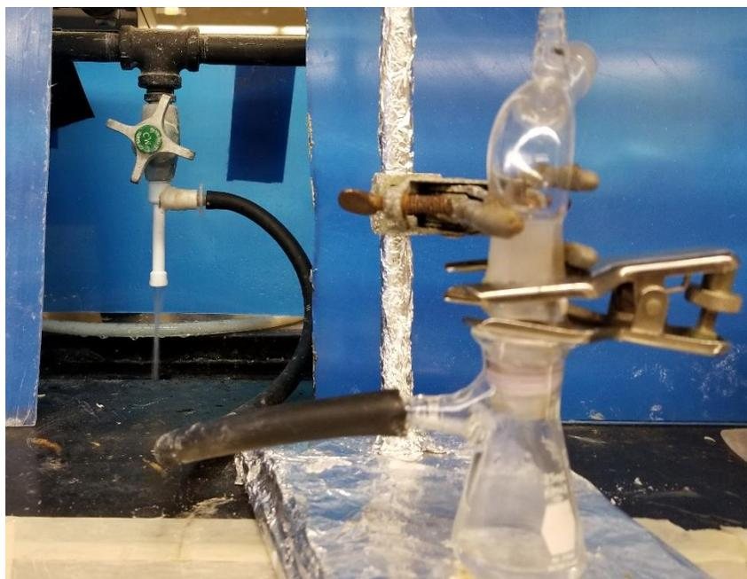
**Figure 13.** NaCl filtration set-up with tap to maintain differential pressure
