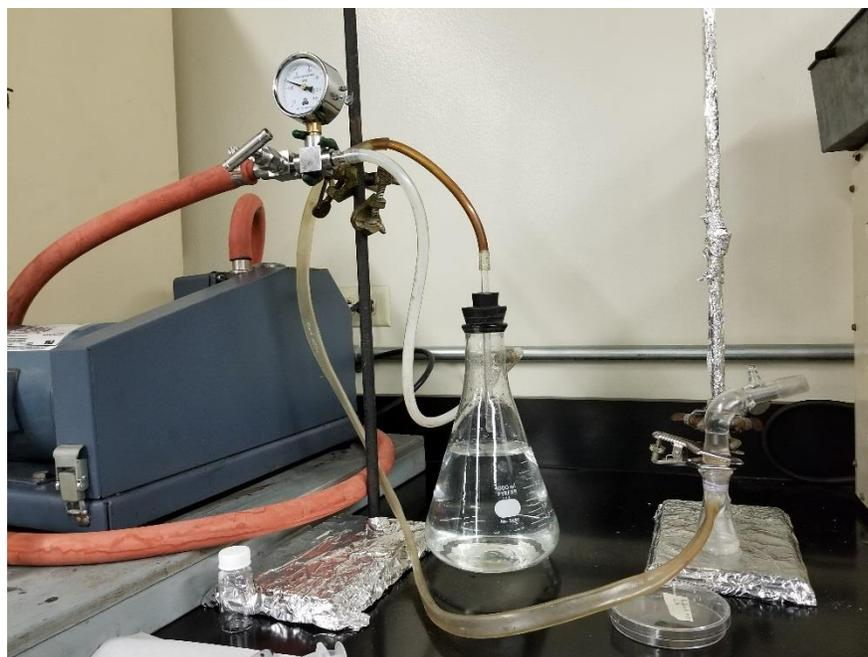
**Figure 12.** NaCl filtration set-up with vacuum pump
