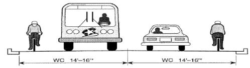
Figure 3.3 Typical Roadway Section With Wide Curb Lanes
