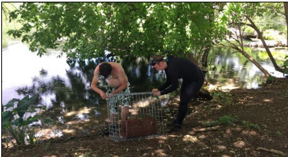
Figure 14. Field assembly of a caged-fish device, with one fish cage.
