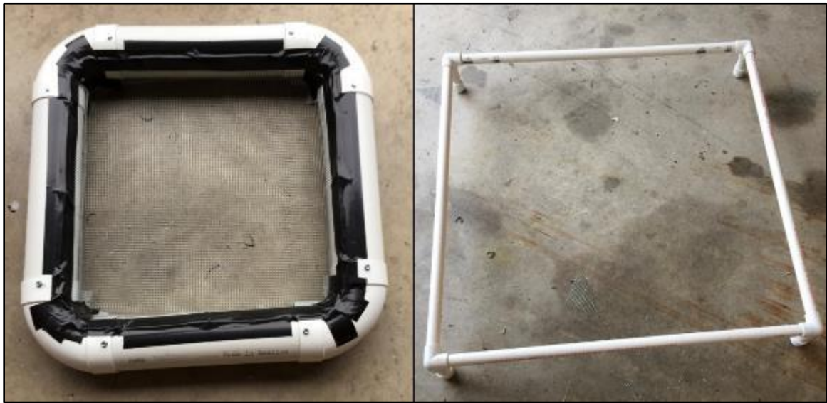
Figure 16. A 1 m X 1 m snail density frame.
