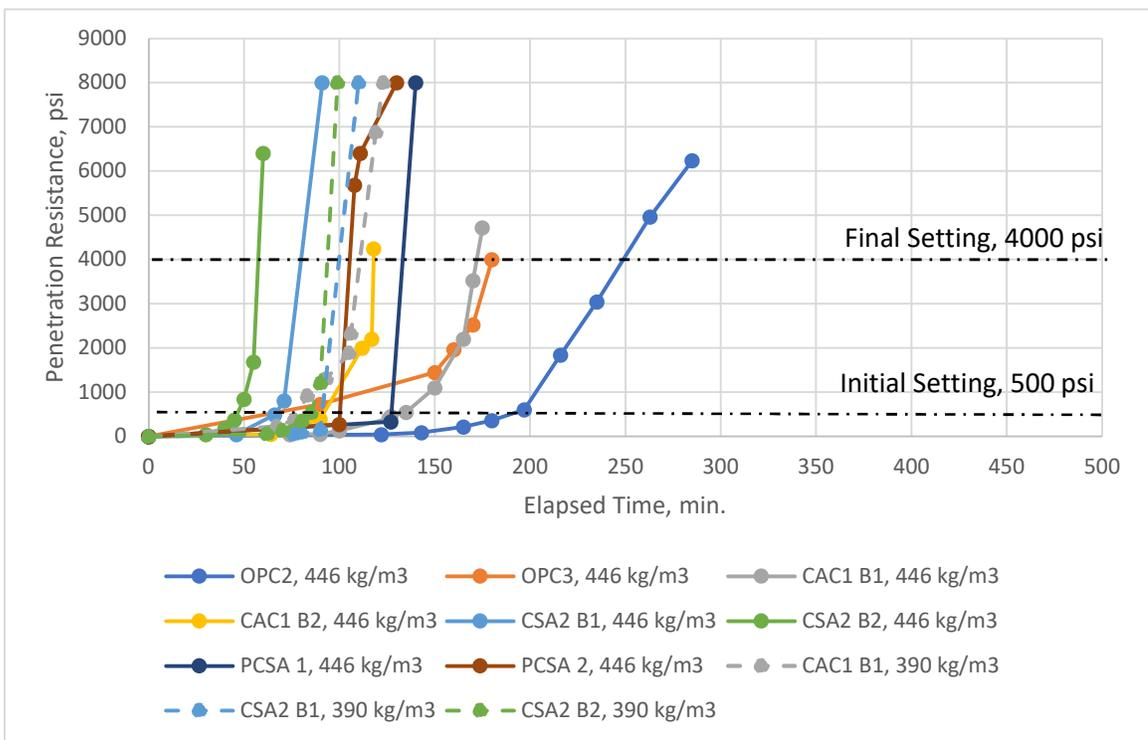
Fig. 5 Setting time of proprietary cement mortar.
