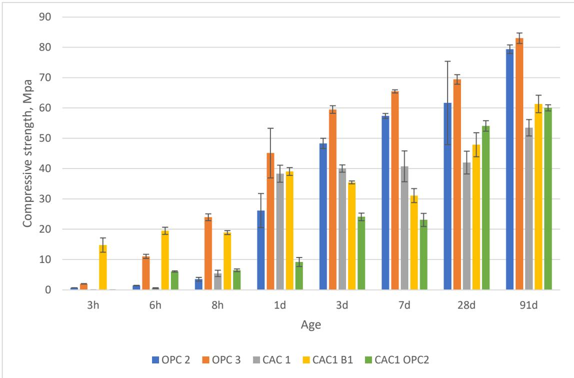
Fig. 10 Compressive strength of CAC cement at 390 kg/m<sup>3</sup> cement binder.
