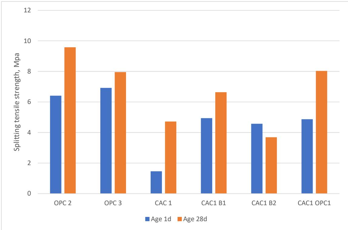
Fig. 13 Splitting tensile strength of OPC 2, 3, CAC cement at 446 kg/m<sup>3</sup> cement binder.
