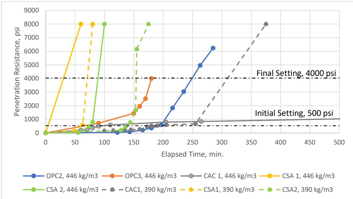
Fig. 4 Setting time of straight cement mortar.
