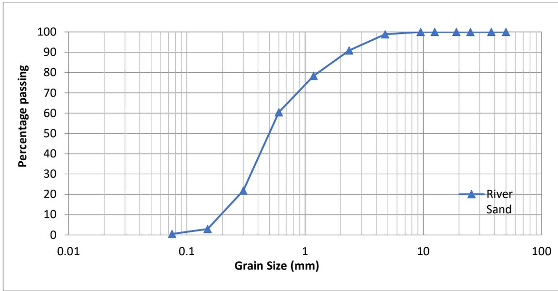
Fig. 3 Sieve Analysis for River sand.
