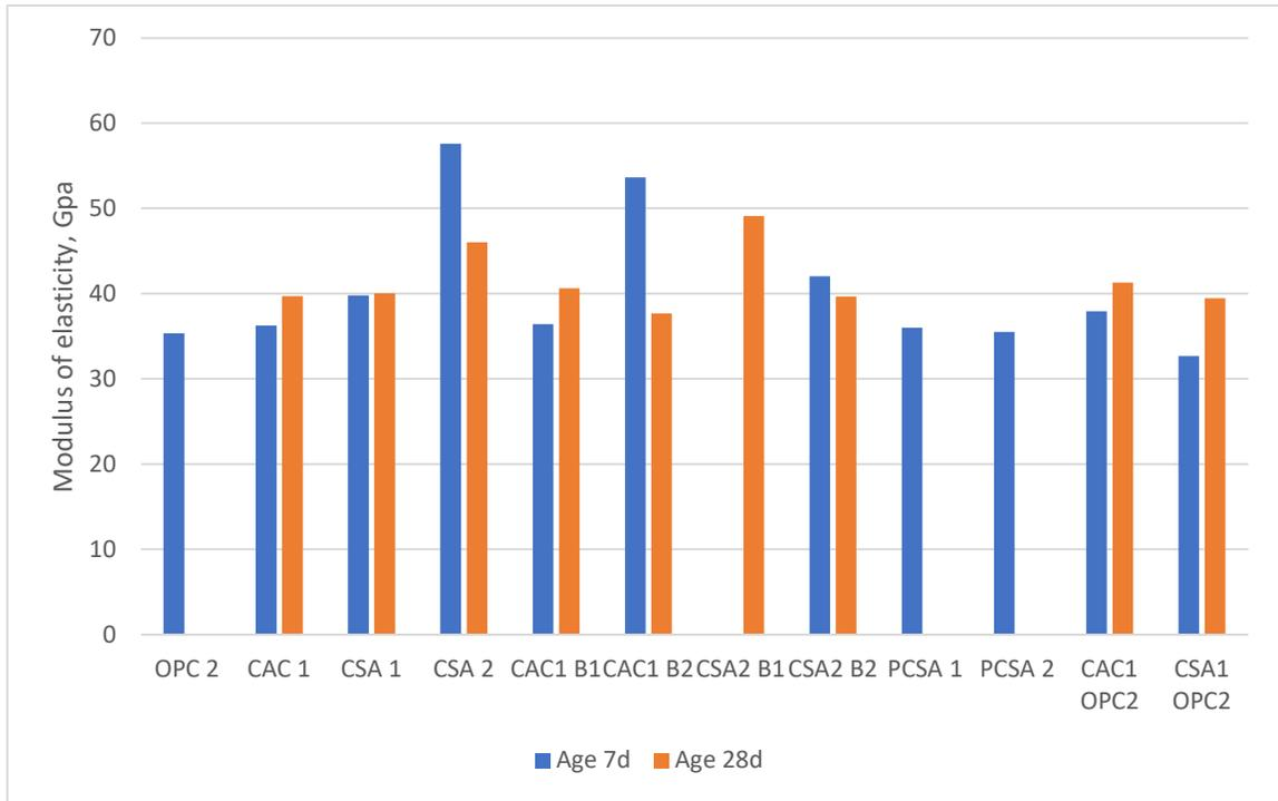
Fig. 17 Modulus of elasticity for concrete mixtures at 446 kg/m<sup>3</sup> cement binder.
