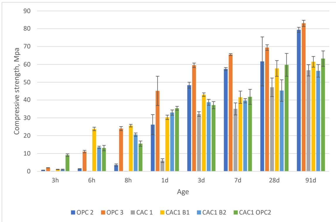
Fig. 7 Compressive strength of CAC cement at 446 kg/m<sup>3</sup> cement binder.
