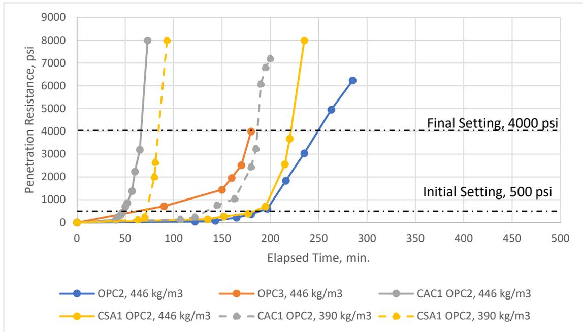
Fig. 6 Setting time of lab-blended cement mortar.
