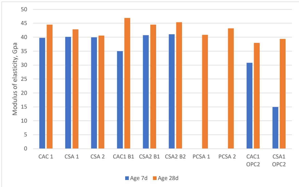
Fig. 18 Modulus of elasticity for concrete mixtures at 390 kg/m<sup>3</sup> cement binder.
