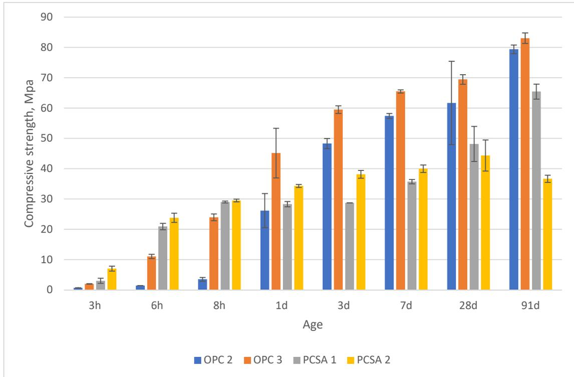
Fig. 12 Compressive strength of PCSA cement at 390 kg/m<sup>3</sup> cement binder.
