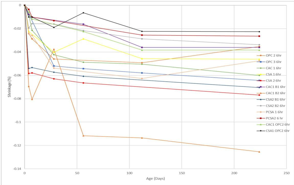
Fig. 19 Drying shrinkage of prism demolded at 6h at 446 kg/m<sup>3</sup> cement binder.
