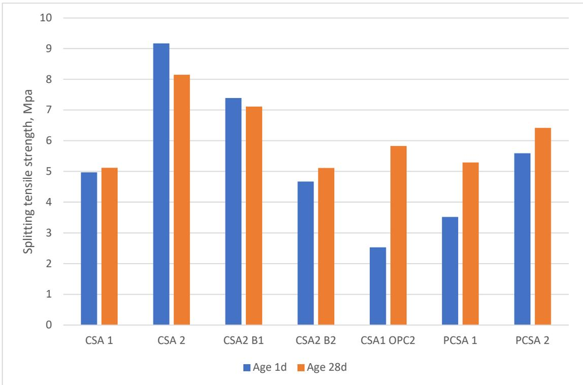
Fig. 14 Splitting tensile strength of CSA cement at 446 kg/m<sup>3</sup> cement binder.
