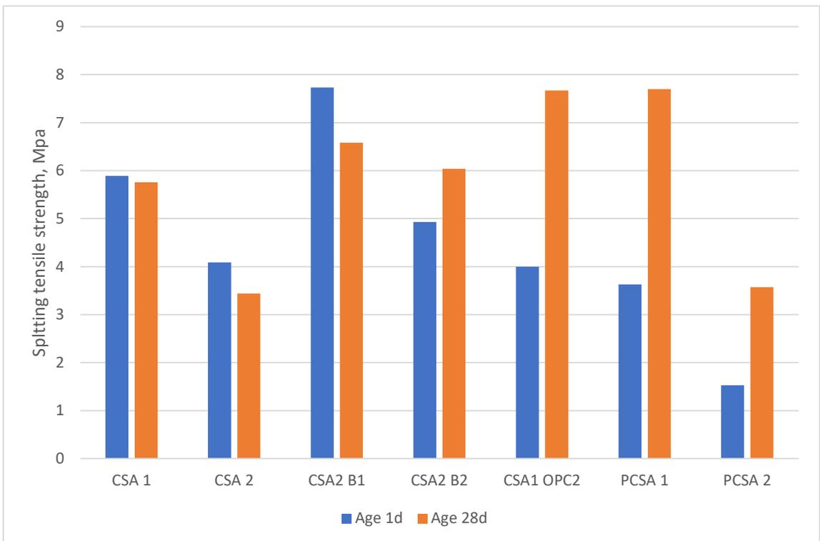
Fig. 16 Splitting tensile strength of CSA cement at 390 kg/m<sup>3</sup> cement binder.
