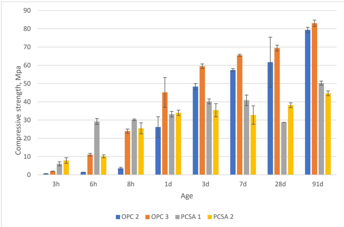
Fig. 9 Compressive strength of PCSA cement at 446 kg/m<sup>3</sup> cement binder.
