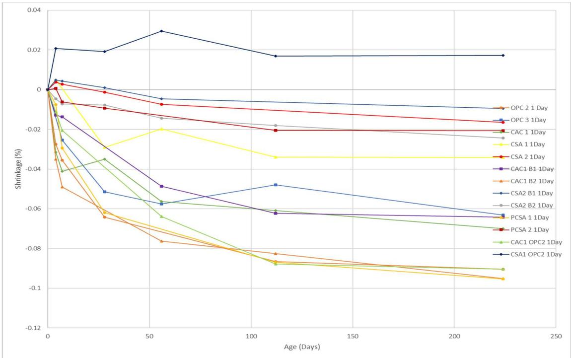
Fig. 20 Drying shrinkage of prism demolded at 1d at 446 kg/m<sup>3</sup> cement binder.
