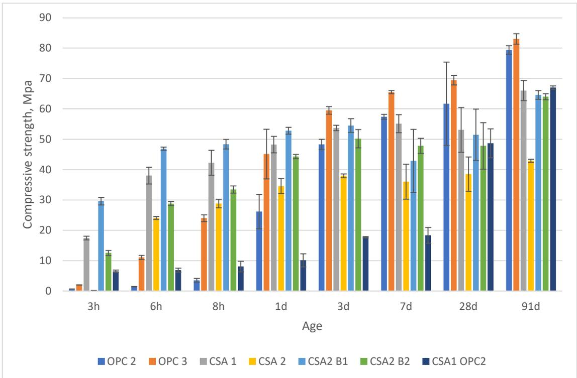
Fig. 11 Compressive strength of CSA cement at 390 kg/m<sup>3</sup> cement binder.
