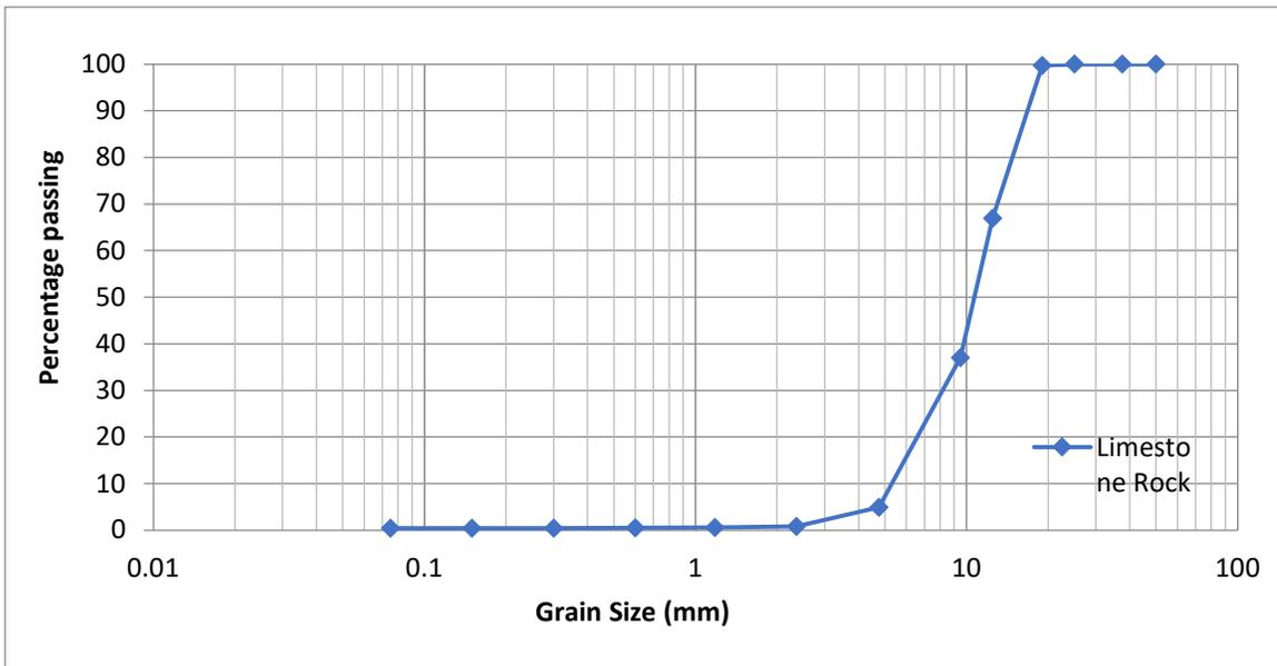
Fig. 2 Sieve Analysis for Limestone Rock.
