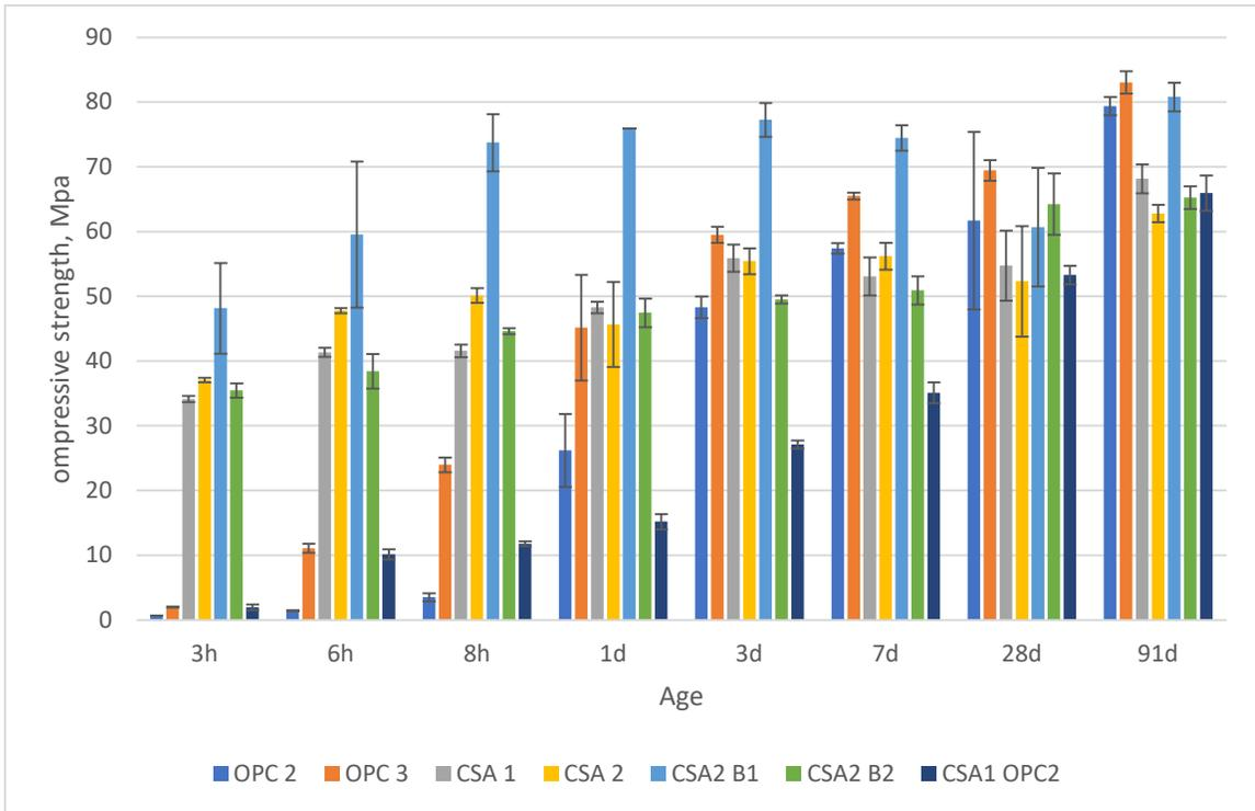
Fig. 8 Compressive strength of CSA cement at 446 kg/m<sup>3</sup> cement binder.
