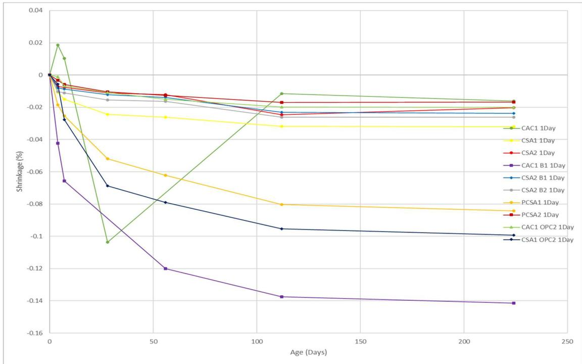
Fig. 22 Drying shrinkage of prism demolded at 1d at 390 kg/m<sup>3</sup> cement binder.
