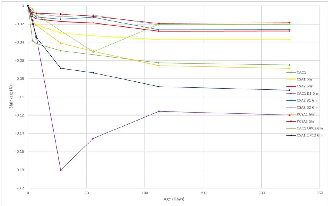
Fig. 21 Drying shrinkage of prism demolded at 6h at 390 kg/m<sup>3</sup> cement binder.
