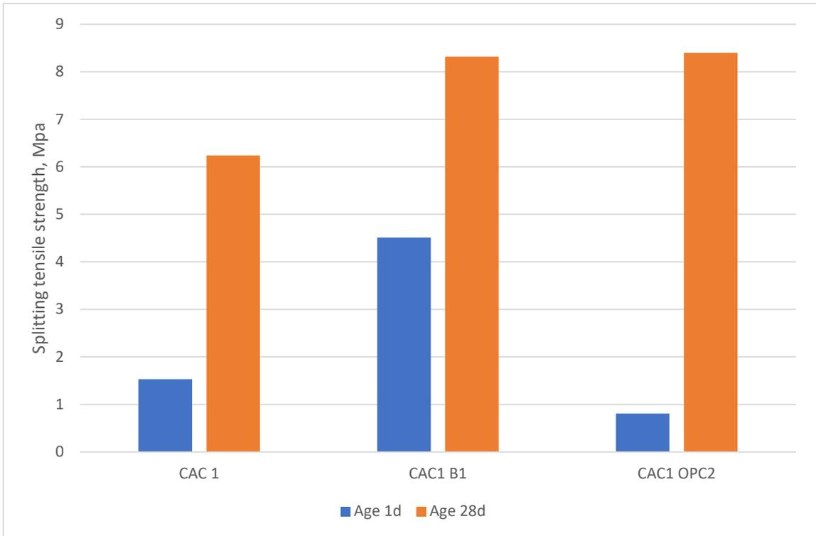
Fig. 15 Splitting tensile strength of CAC cement at 390 kg/m<sup>3</sup> cement binder.
