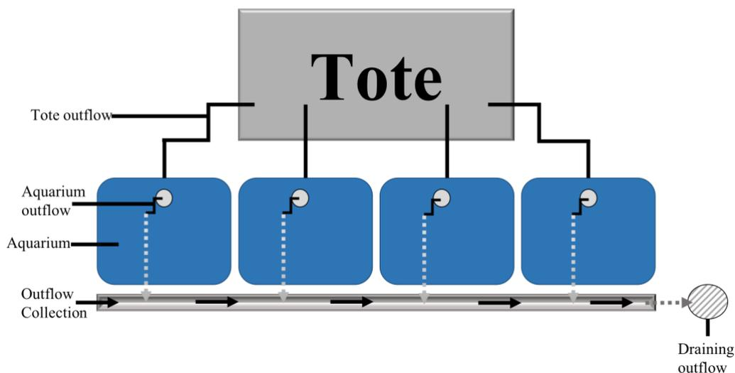
**Figure 2. Continuous aquarium system for chronic nitrite exposure in goldfish.** Totes were filled with water with appropriate nitrite concentrations, aquariums were gravity feed with water from the tote. Valves were used to calibrate rate of tote outflow. Aquarium outflow drained into outflow collection which ultimately drained into Texas State University Freeman building sewer system.
