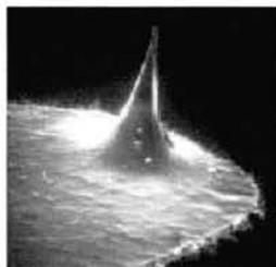
**Figure 2.2 A magnified view of a typical probe used in the AFM.**
