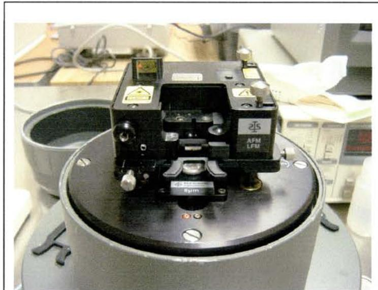
**Figure 2.1 The Atomic Force Microscope.**
