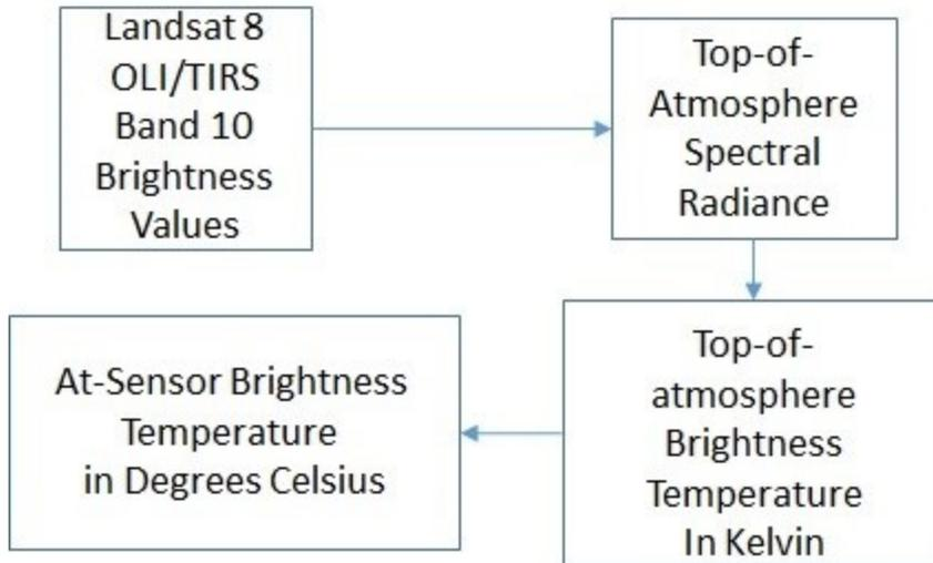
Figure 2: A visualization of the model used to convert Level 1T Data from Landsat to at-sensor brightness temperatures in degrees Celsius.
