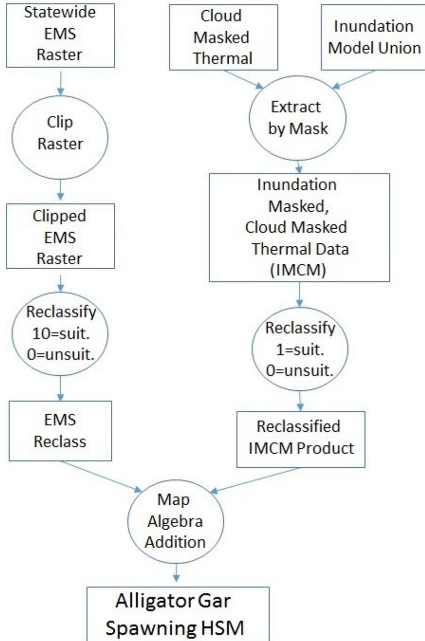
Figure 3: Graphical depiction of HSM workflow. “EMS” stands for Ecological Mapping System and denotes land cover. “IMCM” stands for Inundation-Masked Cloud-Masked product combining thermal and inundation suitability layers. Note that non-inundated
