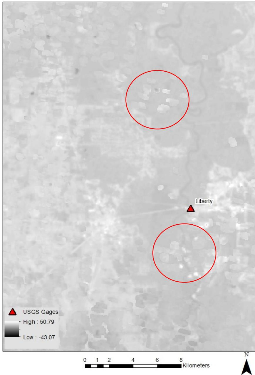
Figure 5: The interim thermal data product before being clipped. The red circles highlight patches of different land surfaces temperatures which represent artifacts of the MINUR process.
