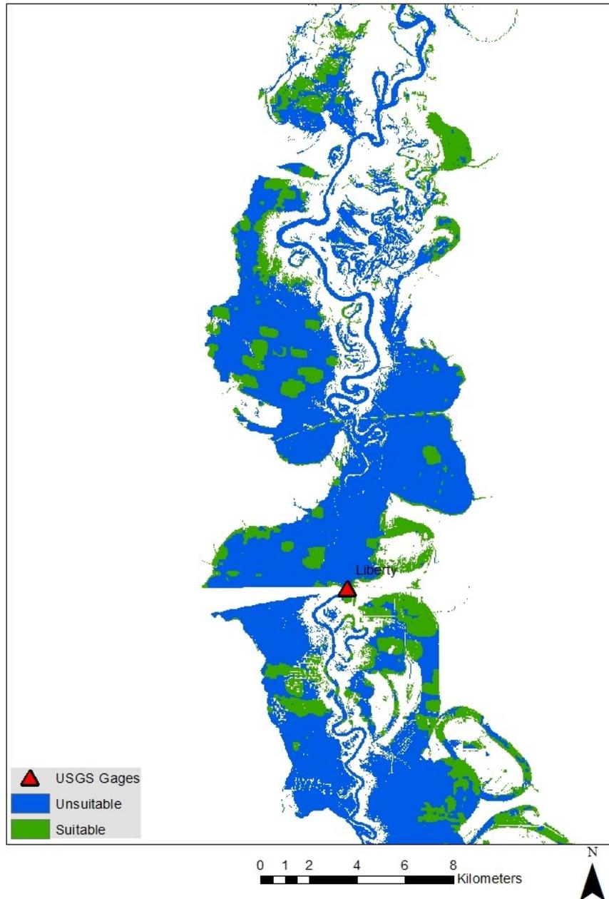
Figure 19: Thermal suitability anomalies for 06 June 2016. Green patches are examples of cloud-generated anomalies in thermal data after replacement of cloud-masked pixels using the MINUR approach.
