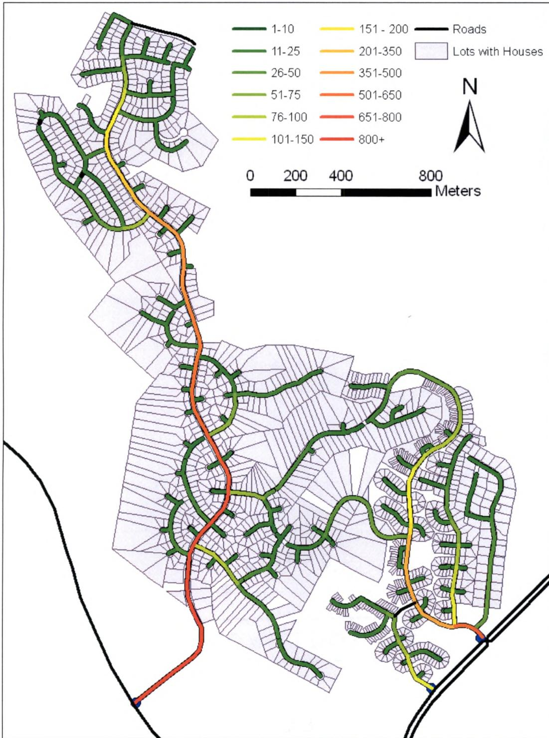
Figure 53. CFA Projected Egress Traffic Distribution: Jester Estates.
