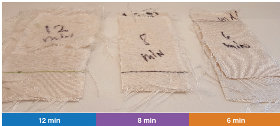
Figure 10. Timing test on woven silica.
