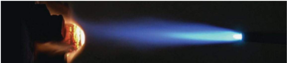
Figure 18. Sample being tested on the oxyacetylene test bed.
