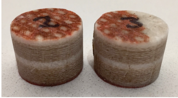
Figure 19. Needle-punched ablation samples.
