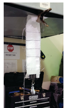
Figure 8. Simple lap-shear test.
