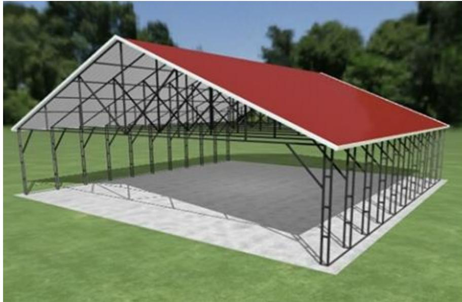
Figure 22: 40' × 40' Vertical-Roof Carport [130]
