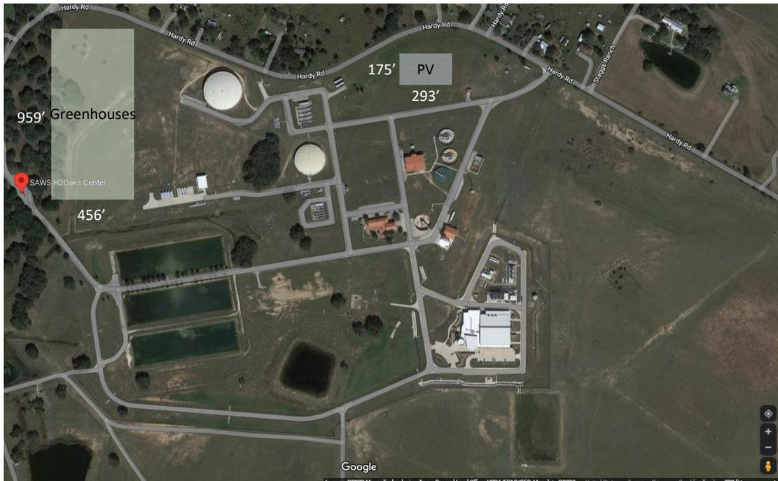
Figure 44: Estimated Footprint of a Full-Scale PBR-Secondary RO Facility with PV in the Sunlight System of 1.5 Days HRT Scenario within the Property of an Existing Brackish Groundwater Desalination Facility in Texas (Source: Google Maps)
