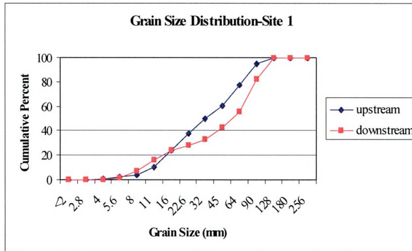
**Figure 25: Comparison of grain size distribution at Site 1.** Average grain size at Site 1A (upstream) is finer than at Site 1B (downstream).
