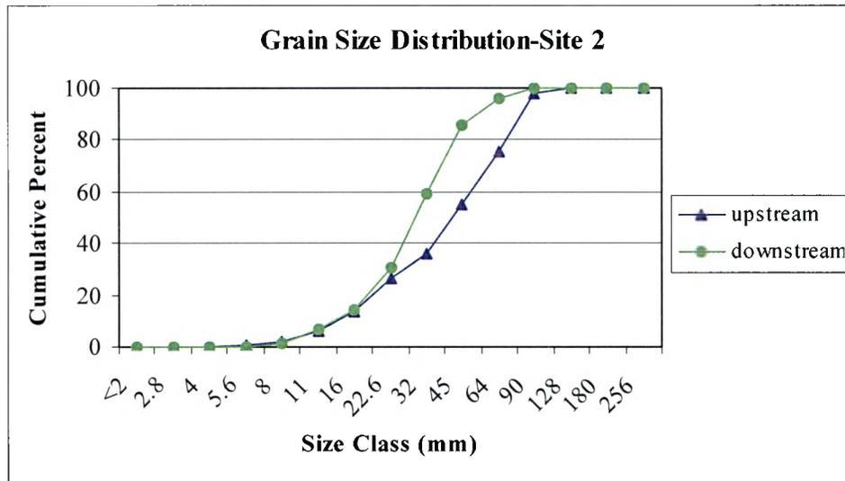
**Figure 30: Comparison of grain size distribution at Site 2.** Average grain size at Site 2A (upstream) is coarser than at Site 2B (downstream).
