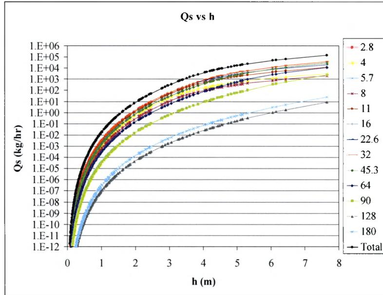
**Figure 39: Sediment transport rates compared to depth over gravel bar at Site 3B.** Transport rates are divided by size class.
