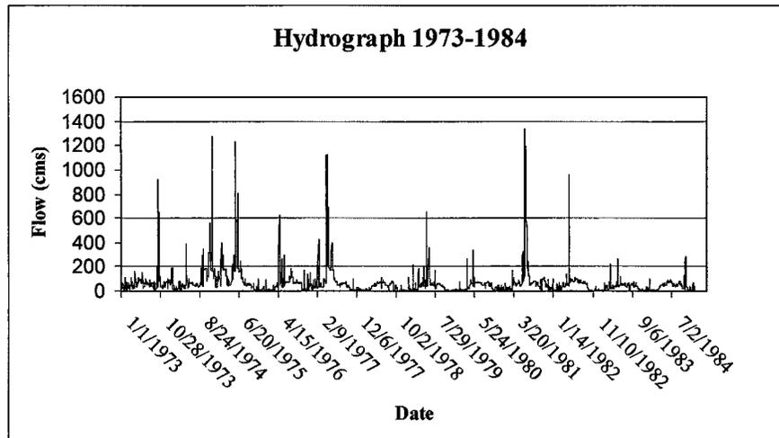
**Figure 7: Hydrograph from 1973-1984.** Several high flow events that likely caused the channel avulsion are observed in this hydrograph. Peak flow (based on USGS gauge data at Bastrop) during these years did not reach the levels that caused the 1991 avulsion, but were significant enough to have induced modifications to the river, either in one event, or over the course of several events.
