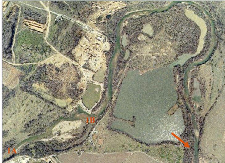
**Figure 17: Approximate location of breach downstream of Site 1.** The red arrow shows the location of the breach between a large pond and the main channel. From Google Earth version 3.0.0762.0.
