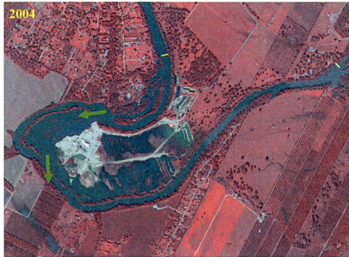
**Figure 21: Image of the gravel mine at Site 3 inundated during a flood in late November 2004.** Flows reached 1068 cms at the Austin gauge (upstream of site) and 1537 cms at the Bastrop gauge (downstream of site). From USDA National Agriculture Imagery Program 2004.
