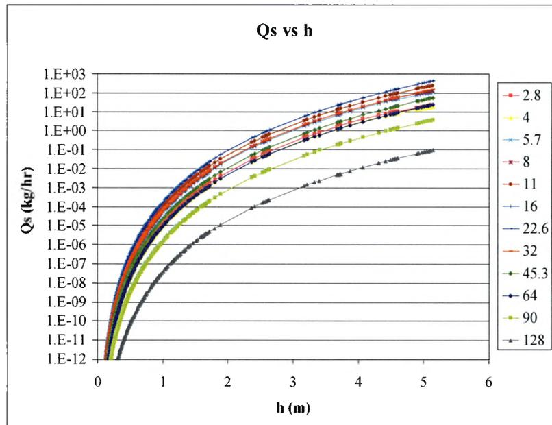
**Figure 26: Sediment transport rates compared to depth over gravel bar at Site 1A.** Transport rates are divided by different size classes.
