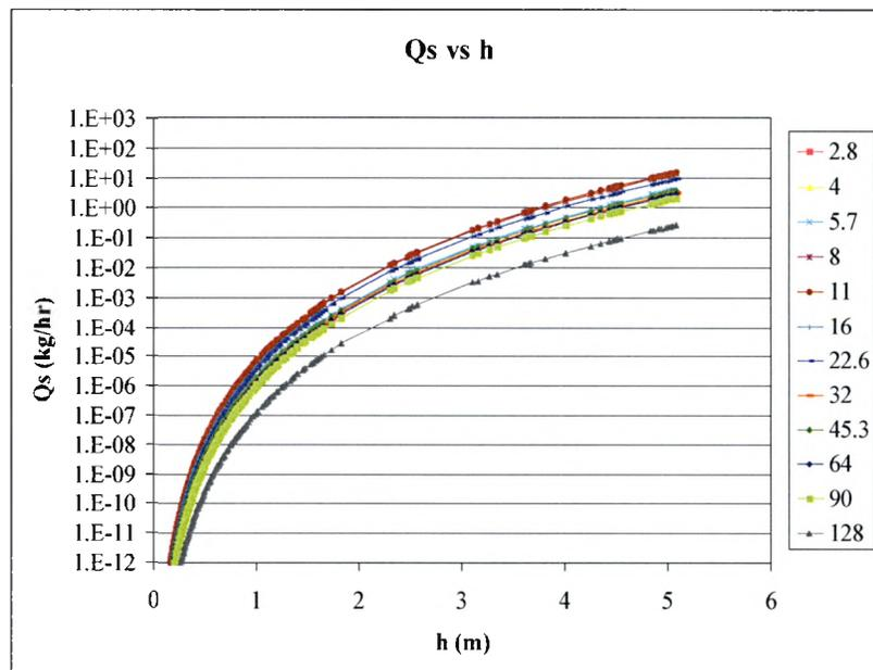
**Figure 28: Sediment transport rates compared to depth over gravel bar at Site 1B.** Transport rates are divided by different size classes.
