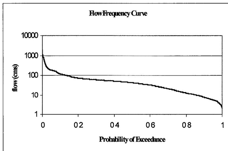
**Figure 3: Flow frequency curve based on USGS data from the Bastrop gauge.** Data ranges between 1960 and 2006, and shows the discharge associated with the 1991 flood to be the highest on record since dam construction.
