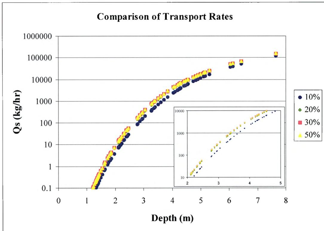
**Figure 40: Sediment transport rates based on percent sand on the channel bed for Site 3B.** Note the increase in movement between 10% sand and higher percentages (20% to 50%) on the bed surface.
