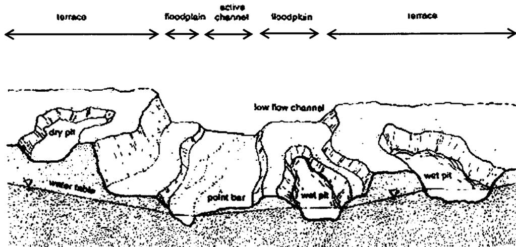
**Figure 15: Schematic of various mining methods.** Notice the proximity to the active channel and the water table. From Kondolf (1994a).
