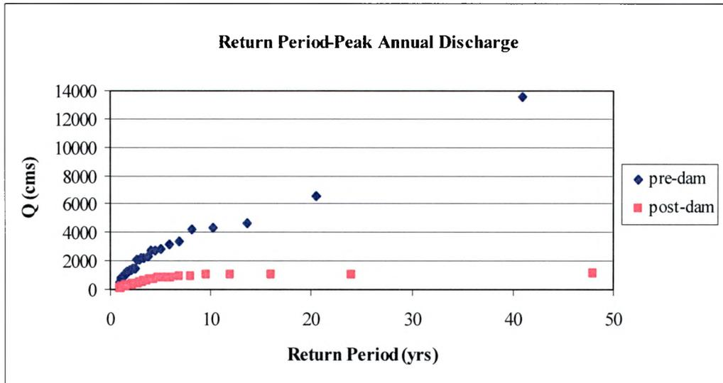
**Figure 14: Return period and corresponding magnitude of flows.** A comparison of annual discharge prior to dam construction (1898-1937) and following dam construction (1960-2006), based on USGS gauge data at Austin.
