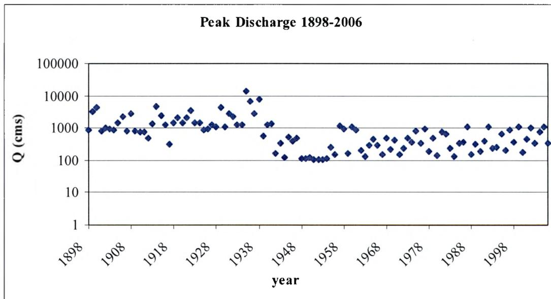
**Figure 13: Peak annual discharge from 1898-2006.** Note the dramatic drop in discharge in the late 1930s (data from USGS gauge at Austin).
