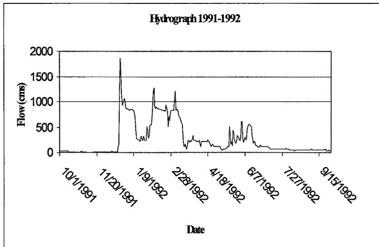
**Figure 4: Hydrograph from USGS data at the Bastrop gauge.** Flows associated with a major flood in late 1991 show discharge rates that exceeded 1800 cms and remained high for six months following from releases of upstream reservoirs. During this time the channel carved a new path.
