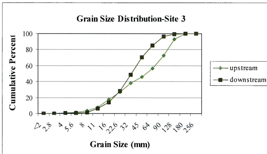
**Figure 36: Grain size distribution of Site 3A (upstream) and Site 3B (downstream).** Average grain size at Site 2A (upstream) is coarser than at Site 2B (downstream).
