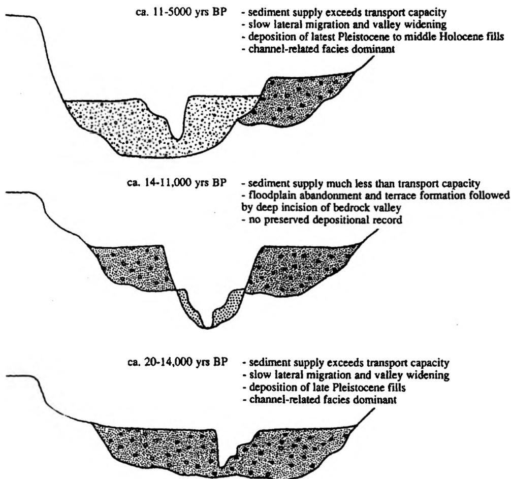
**Figure 10: Schematic of valley cross sections.** The depositional history of late Pleistocene and Holocene alluvial terrace and valley fill is summarized in these cross sections (from Blum 1992).
