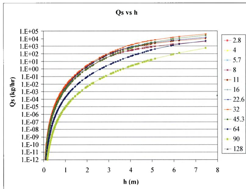
**Figure 33: Sediment transport rates compared to depth over gravel bar at Site 2B.** Transport rates are divided by different size classes.
