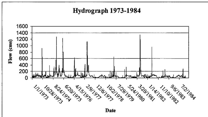
**Figure 7: Hydrograph from 1973-1984.** Several high flow events that likely caused the channel avulsion are observed in this hydrograph. Peak flow (based on USGS gauge data at Bastrop) during these years did not reach the levels that caused the 1991 avulsion, but were significant enough to have induced modifications to the river, either in one event, or over the course of several events.
