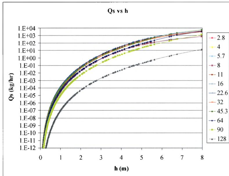
**Figure 31: Sediment transport rates compared to depth over gravel bar at Site 2A.** Transport rates are divided by different size classes.
