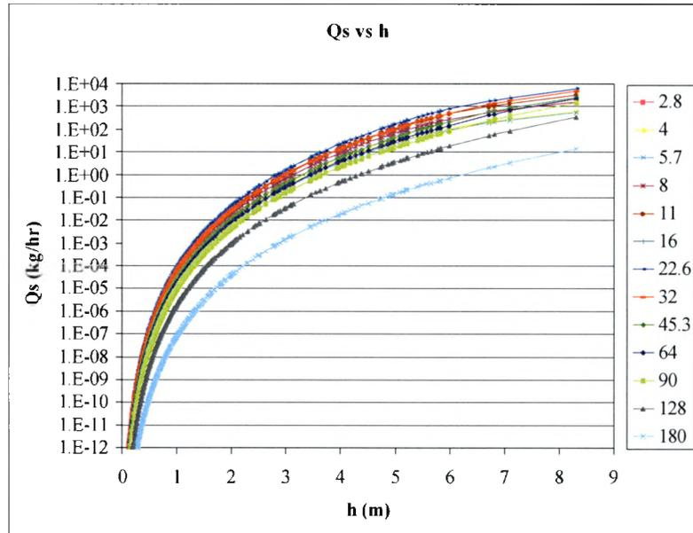
**Figure 37: Sediment transport rates compared to depth over gravel bar at Site 3A.** Transport rates are divided by different size classes.
