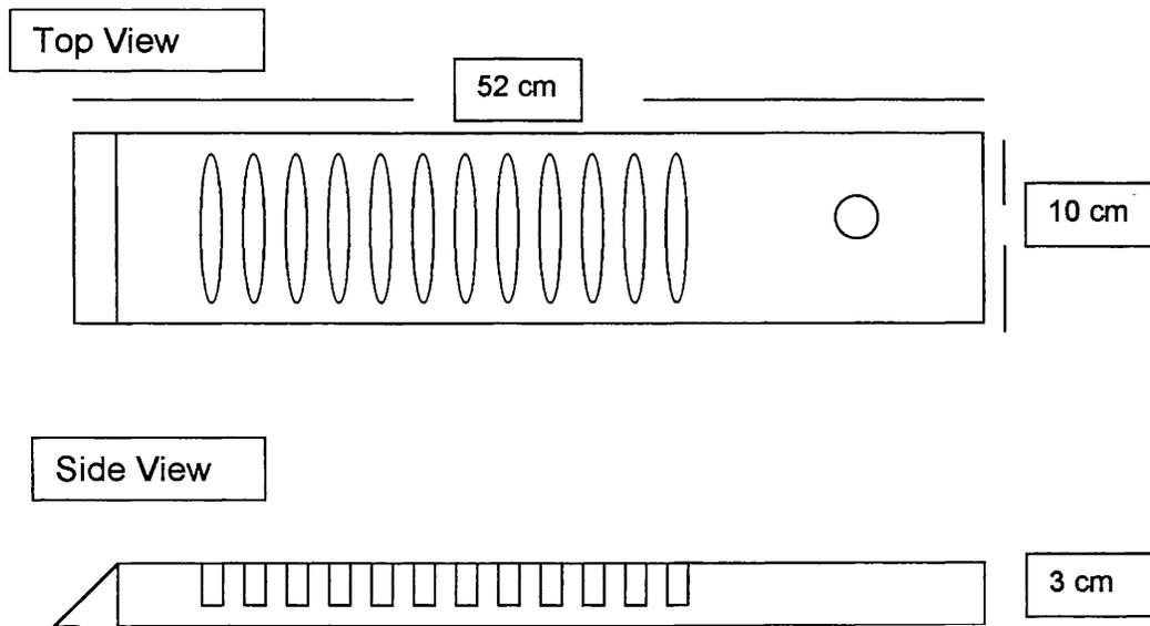
Figure 3. Interstitial water sampler ("peeper").
