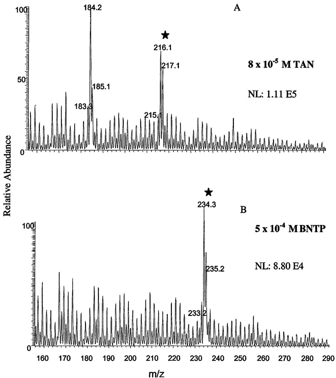
**Fig 3.25 Mass spectra for TAN and BNTP in the PASH matrix.**
