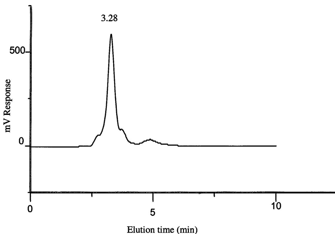
**Fig.3.14 HPLC profile for PASH fraction from Arabian Crude Oil.**
