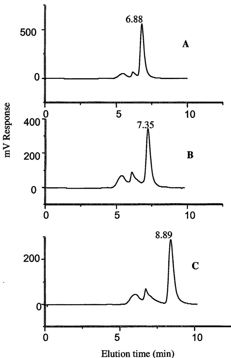
**Fig 3.8. Chromatograms for the organosulfur standard mixture after the addition of: A) 4,6-DBT B) 2-DBT and C) BNTP**
