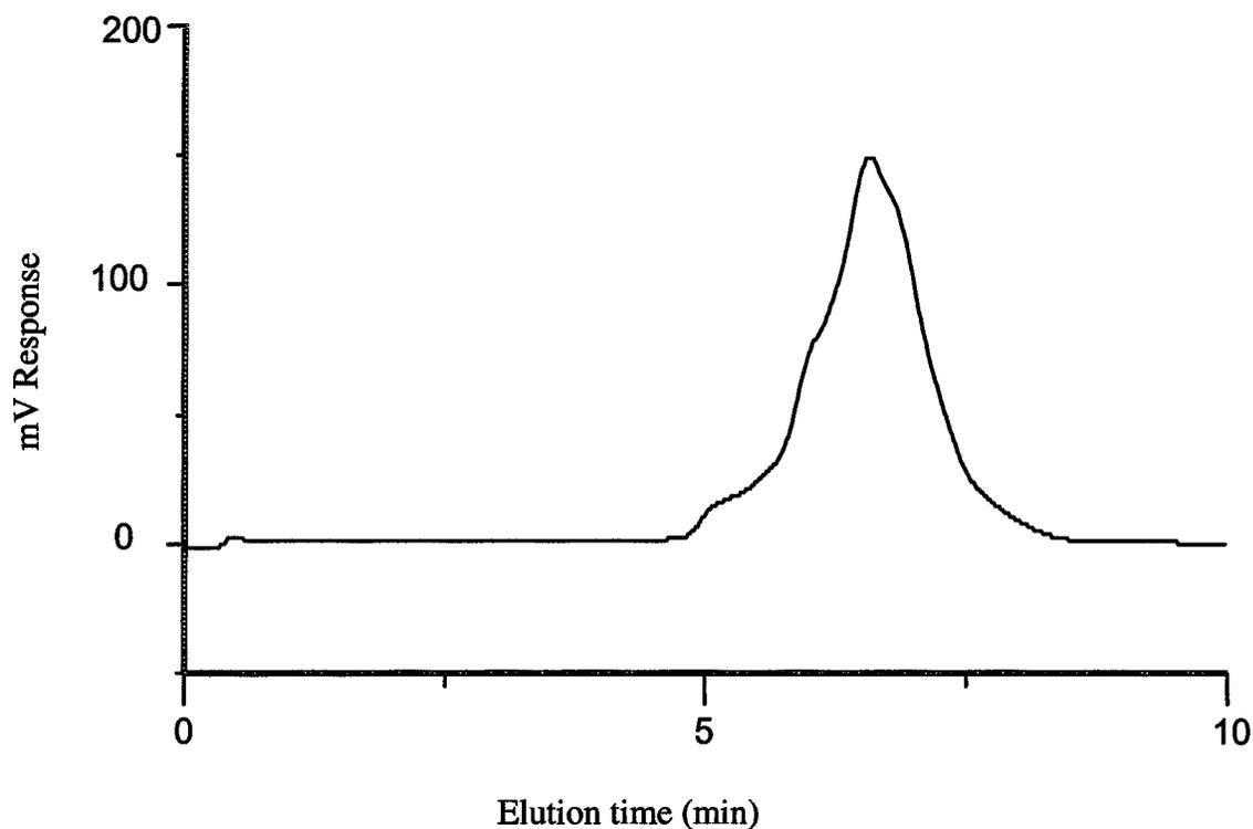
**Fig. 3.16 HPLC of PASH Fraction 2 collected from LC-NH<sub>2</sub> column.**
