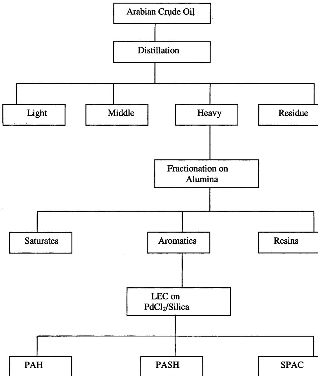
**Fig 2.2 Scheme for the fractionation of the Arabian Crude Oil.**
