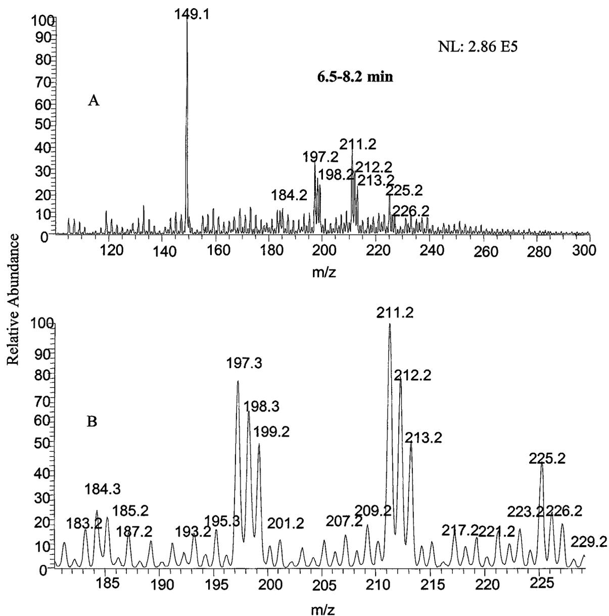
**Fig. 3.17 HPLC/APCI/MS scan of PASH Fraction 1 between 6.5 – 8.2 min.**
