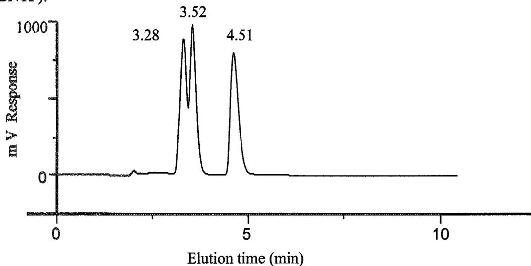
**Fig.3.1 HPLC profile for a mixture of organosulfur compounds.**
