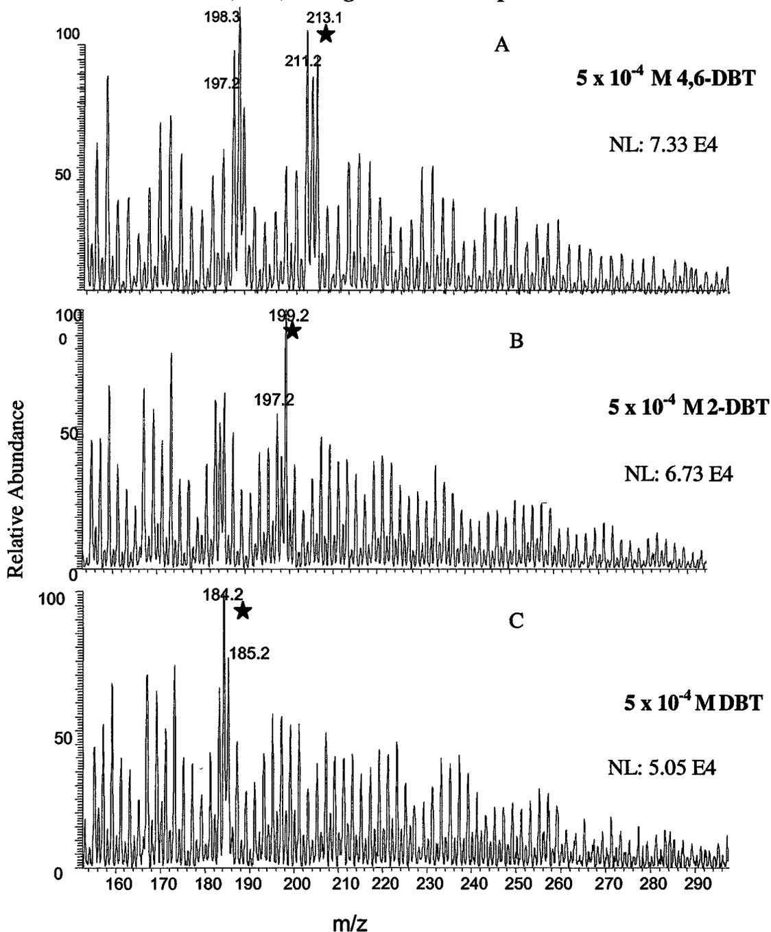
**Fig 3.24** Mass spectra for 4,6-DBT, 2-DBT and DBT in the PASH matrix
