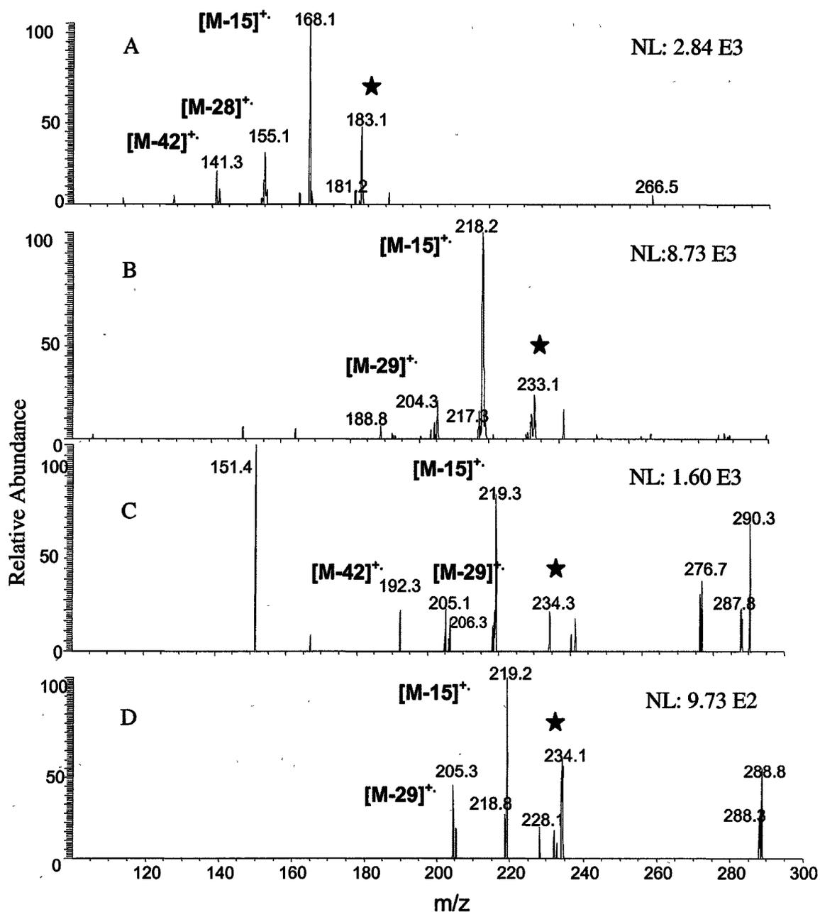
**Fig 3.23 HPLC/APCI/MS<sup>3</sup> for PASH Fraction.**
