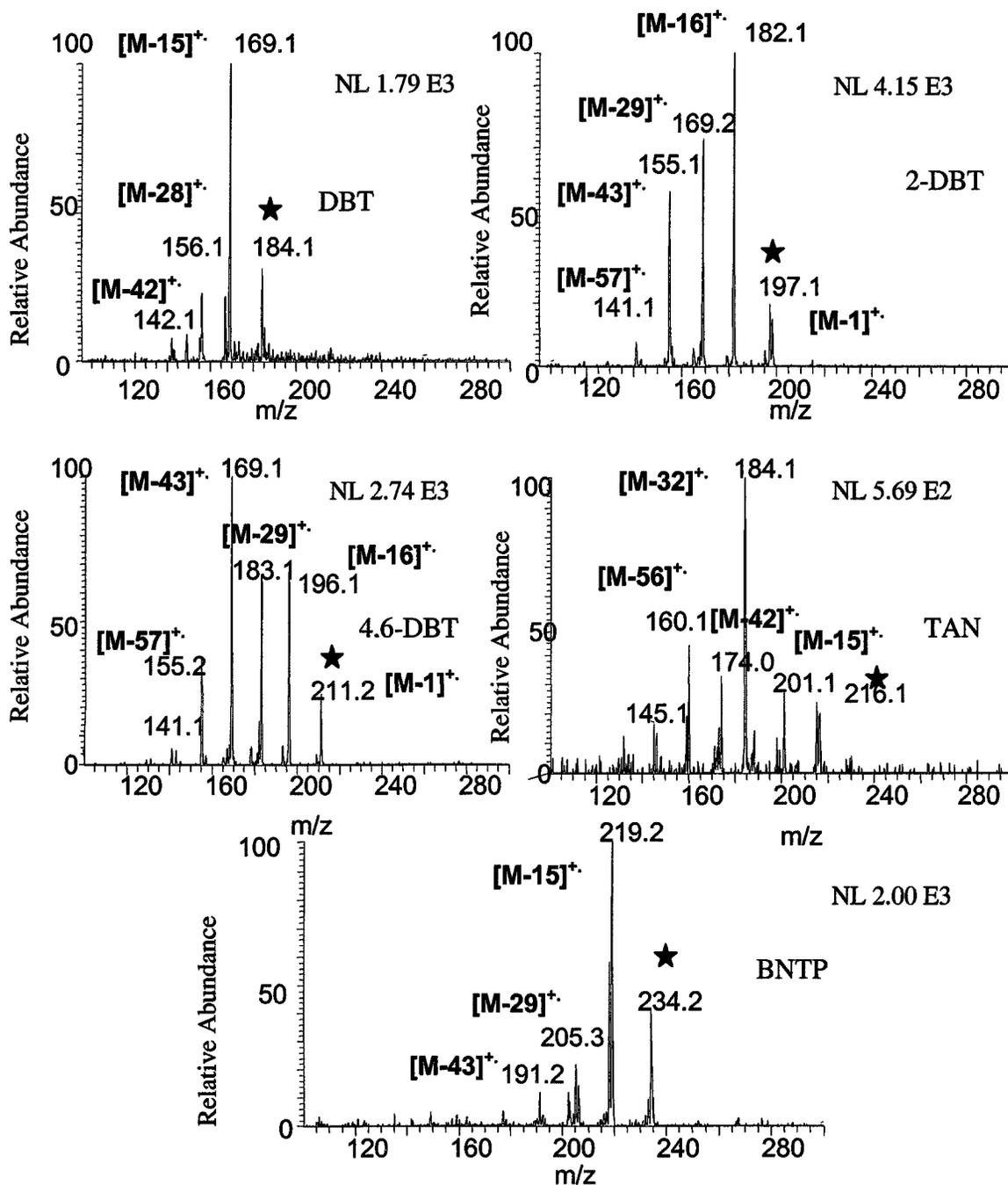
**Fig 3.12 HPLC/APCI/MS/MS for organosulfur standards.** Mobile Phase, hexane:CH<sub>2</sub>Cl<sub>2</sub> (70:30); Flow Rate, 0.3ml/min ; post column addition of 1mM tropylium tetrafluoroborate solution, Flow Rate, 15  $\mu$ l/min. Collision energies are 38, 41, 41, 41, 43% for DBT, 2-DBT, 4,6 DBT, TAN & BNTP respectively.
