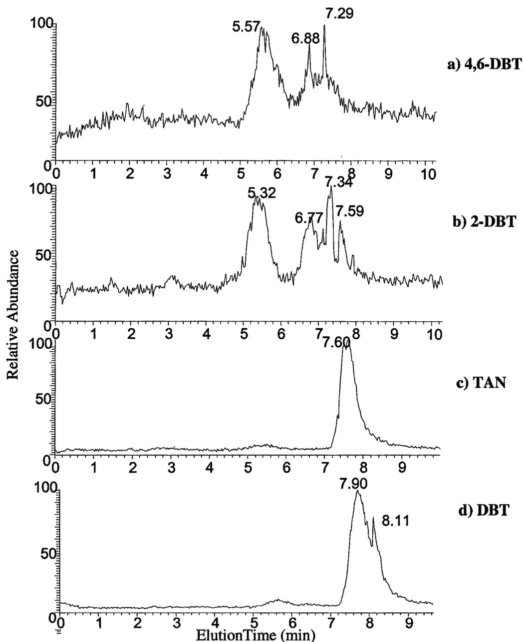
**Fig 3.6 Chromatograms of Fraction 1 showing the elution profile for each of the organosulfur standards.**
