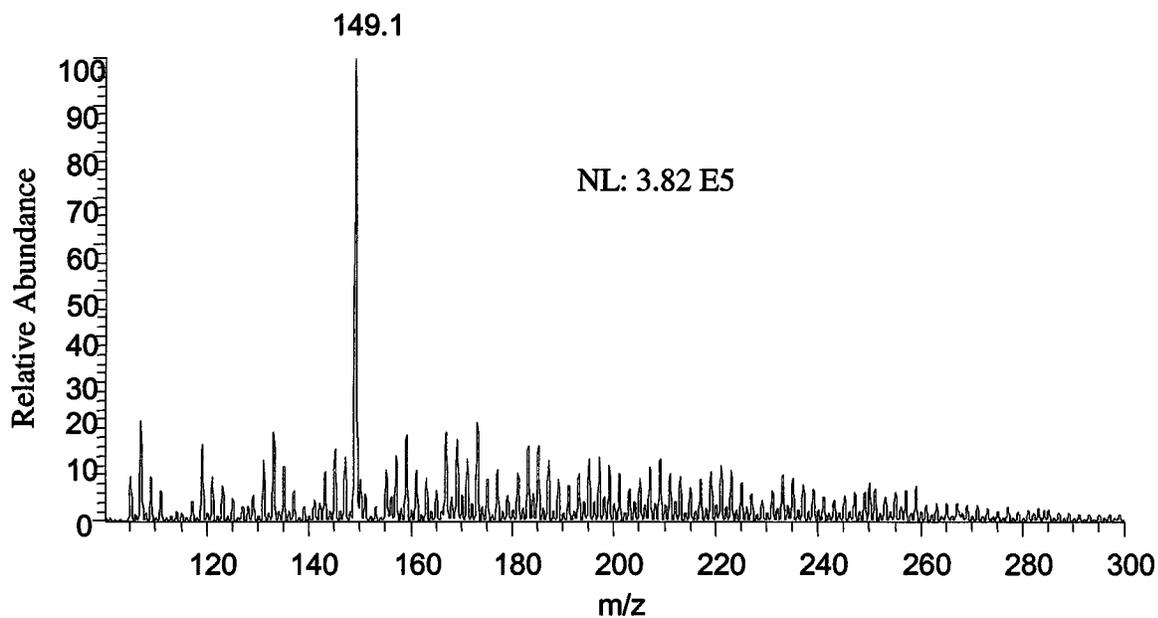
**Fig. 3.5 APCI/MS scan of 1 mM tropylium in full scan mode.**
